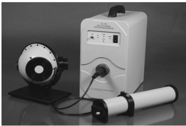
Figure 14.4 Gooch & Housego 6 in. integrating sphere with OL770-LED spectroradiometer. (Source: http://www.ghinstruments.com/products/spectroradiometers/ol-770-led-test-and-measurement-system/ .)
