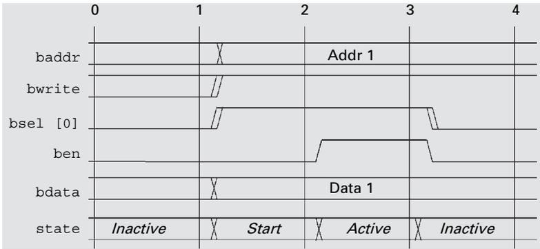
Figure 3.12 Basic write operation
