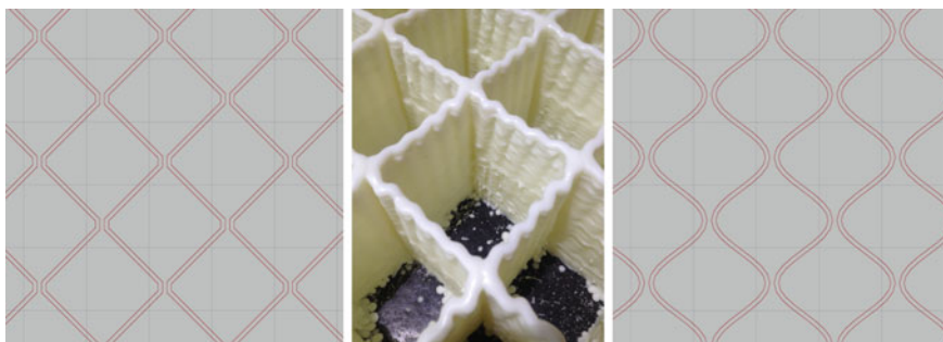
Fig. 5 Square grid internal geometry patten ( left ); wobble visible in the 3D print due to vibrations in the wax extruder head ( centre ); sine wave internal geometry pattern ( right )
