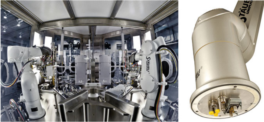
Fig. 3 Stäubli HE robots in a cleanroom environment ( left ), protected interconnection cables for robots in humid or cleanroom environments ( right )
