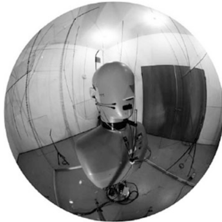
Fig. 3 Measuring acoustic response of a reverberant space using a head and torso simulator
