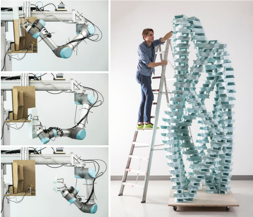
Fig. 16 The robot picks extruded Styrofoam cubes and moves them through the hotwire along a computed path, thus utilizing the robot's potential for performing spatially unrestricted tasks (Gramazio and Kohler, FCL Singapore, 2013, student project by Aejmelaeus-Lindstroem P, Chiang PH and Lee PF)
