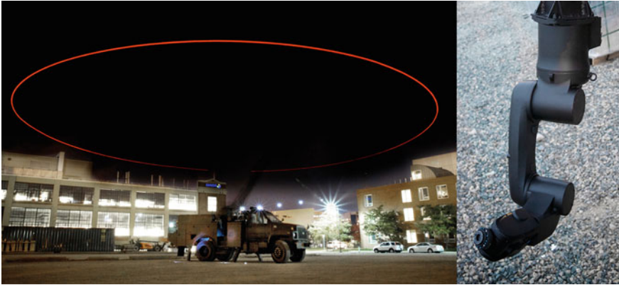
Fig. 2 The range of motion for the DCP is shown through long-exposure photography ( left ). The DCP uses a combination system of a 5-axis Altec hydraulic boom arm and a small 6-axis KUKA robotic arm ( right )
