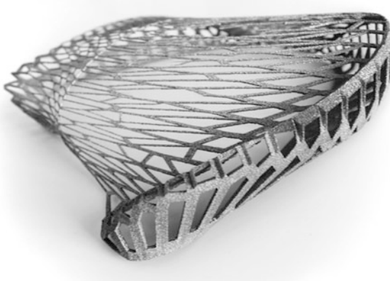
Fig. 1 Procedural lattice: prototype featuring nodes with variable branch count, branch depth and thickness. This hypothetical design for highly articulated structural frame demonstrates effective wire-like branches 1.5 mm thick spanning just over 30 mm
