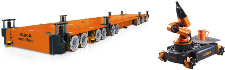
Fig. 3 Up to 90 t payload KUKA omniMove (left), 0.5 kg payload youBot (right)
