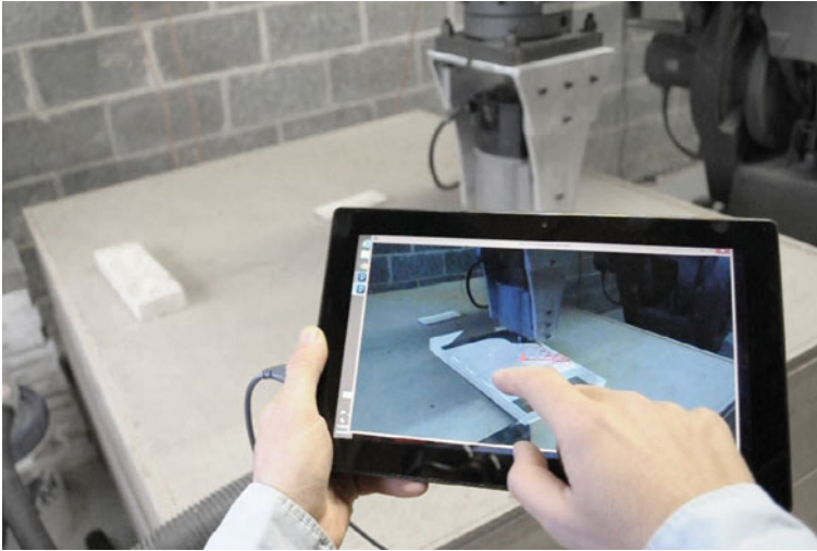
Fig. 2 Toolpaths are displayed on the tablet and can be modified on the fly
