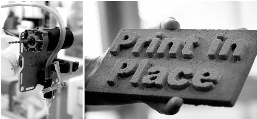
Fig. 5 Combining additive and subtractive processes in a compound end effector ( right ) facilitates fast build times and high resolutions, as seen in the cast structure produced from a printed and milled mold
