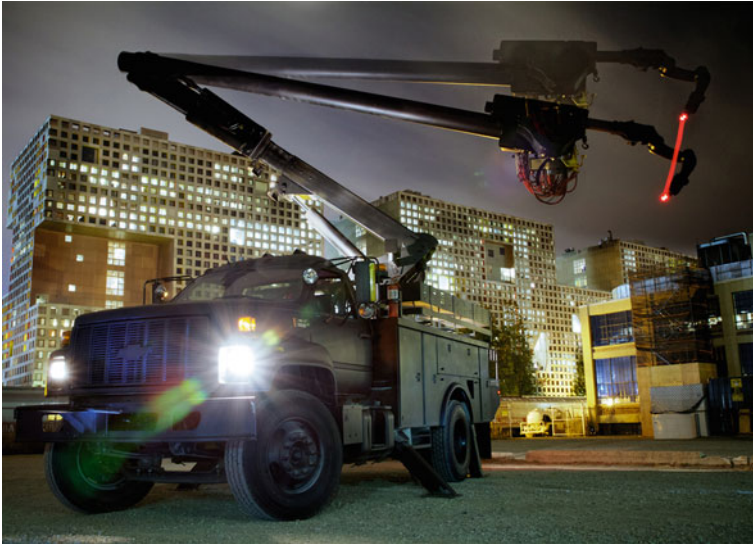
Fig. 1 The digital construction platform (DCP) is comprised of a 6-axis KUKA robotic arm mounted to a 5-axis Altec hydraulic boom arm
