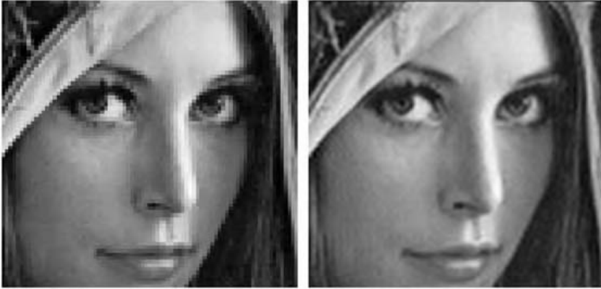
Figure 4. A fragment of the 256 \times 256 pixel test image “Lena” strongly zoomed to reveal the pixel sizes ( on the left ), and its interpolation with CEDCT ( on the right ).
