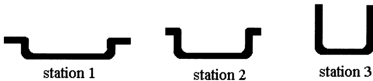
FIGURE 8.9 A three-station drawing operation.
