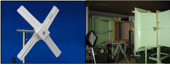
Fig.4 : Corrugated airfoil wind turbine and Goettingen wind tunnel
