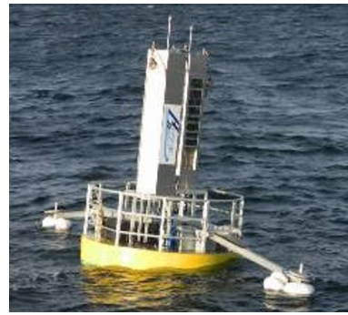
Photo 1: Dielectric Elastomer Generator System on the Buoy Used in December 2008
