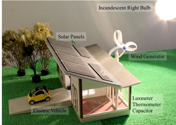
Fig.3: Schematic of SSE Experimental Apparatus (1/24 scale)
