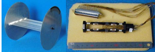
Fig.2: Experimental model and The three-component balance
