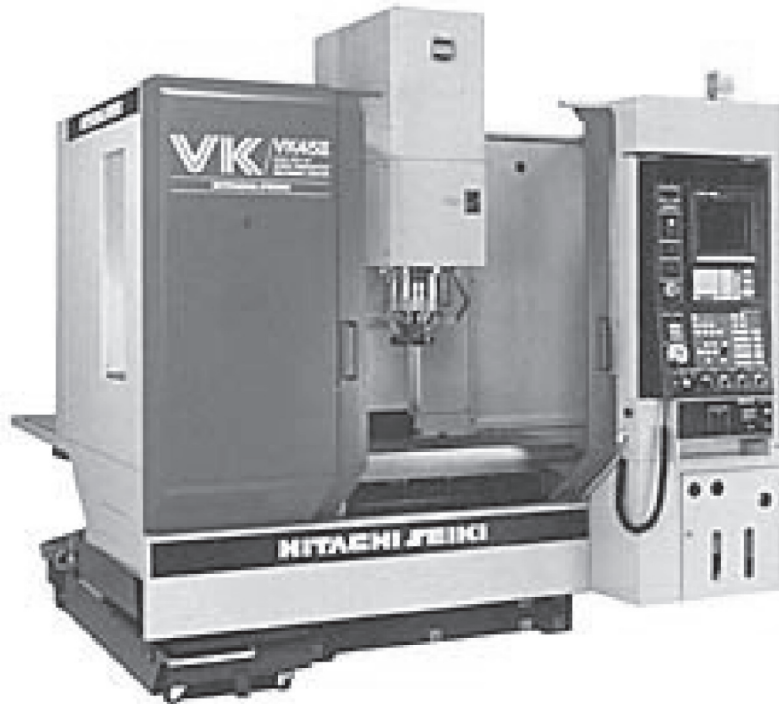
Figure 2.15: A vertical CNC milling machine. Source: Hitachi Seiki Co., Ltd.
