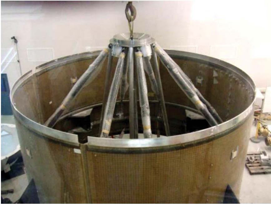
Figure 5-4. Completed struts mounted in the MLAS vehicle. (Courtesy NASA)
