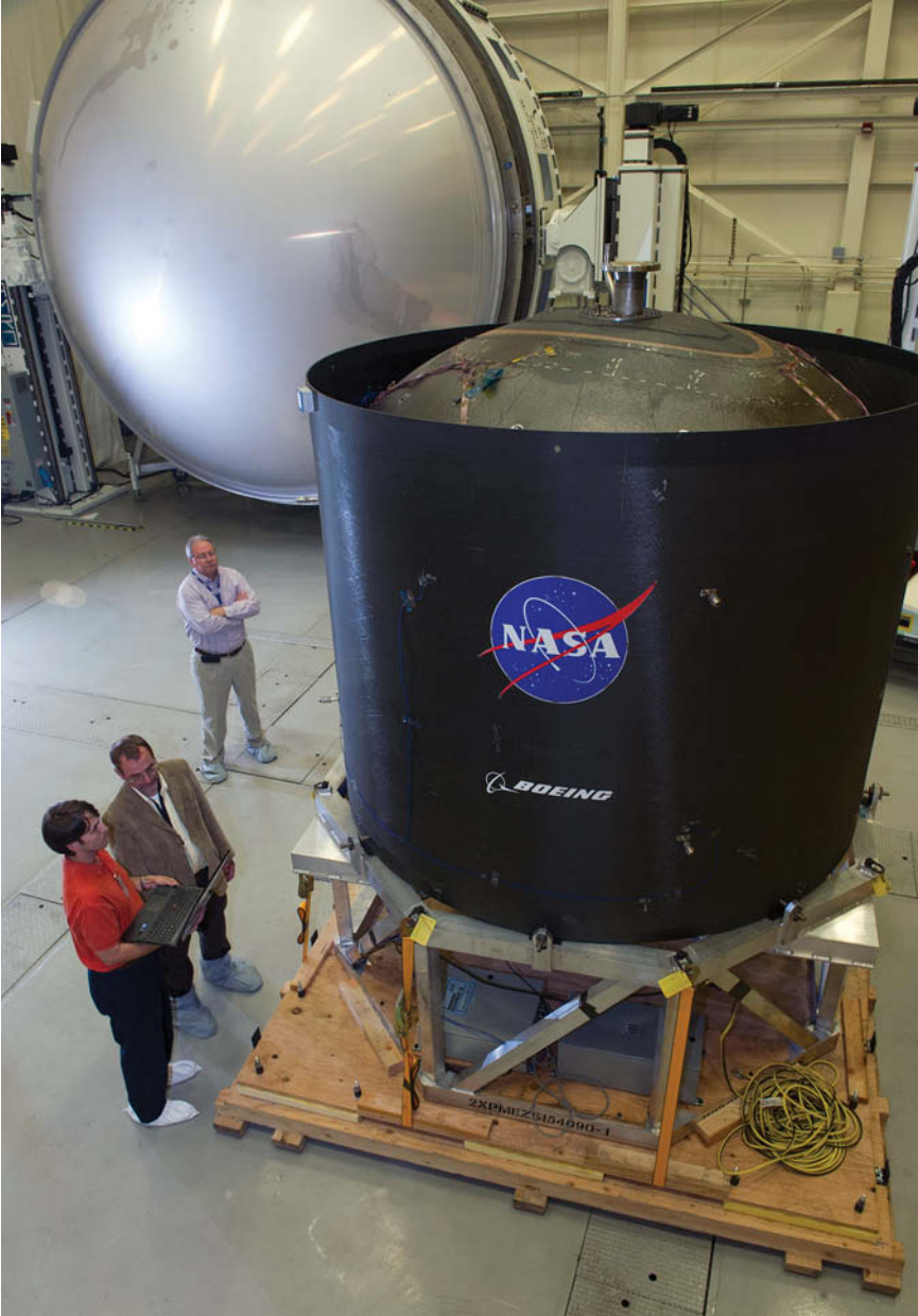
Figure 11-2. NASA's award-winning composite LH 2 cryo-tank. (Courtesy NASA)
