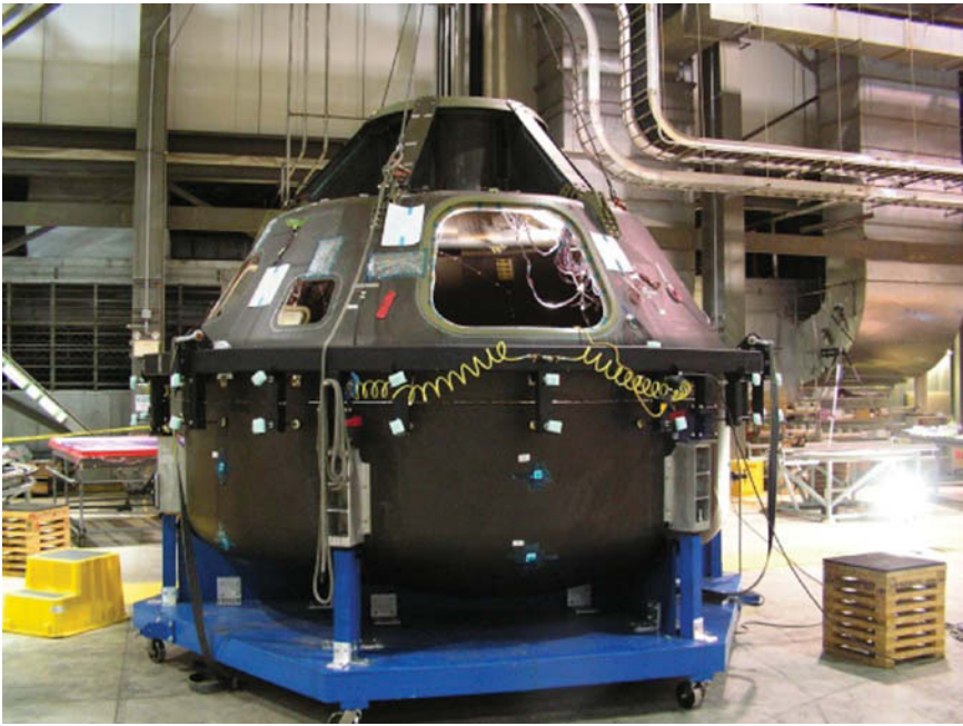
Figure 5-6. Composite crew module. (Courtesy NASA)
