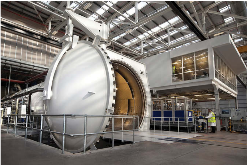
Figure 10-3. Large autoclave for curing aerospace parts.
