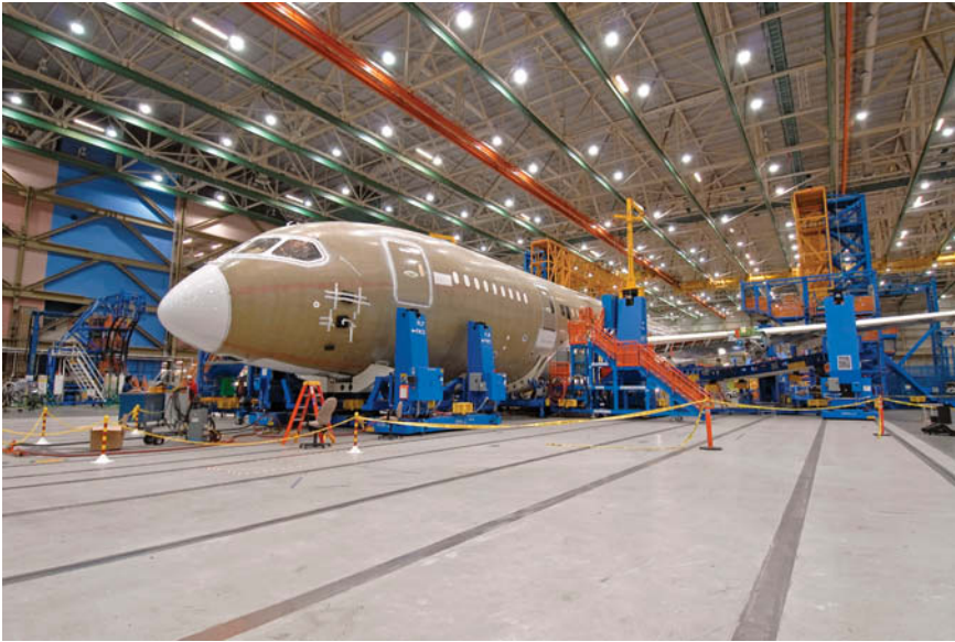
Figure 8-4. Open-architecture assembly line.
