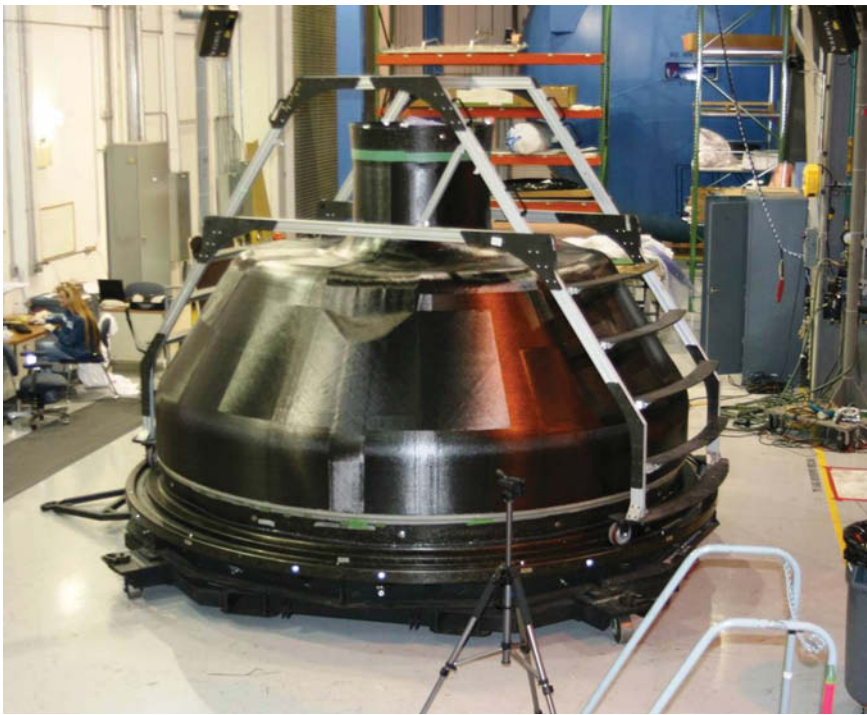
Figure 3-2. Installed parachute fitting. (Courtesy NASA)
