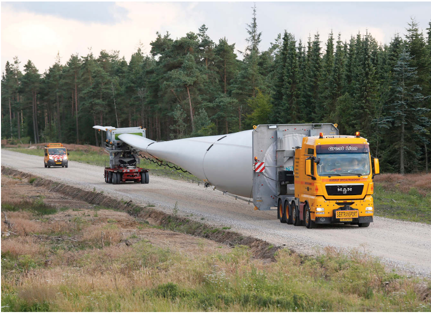
Figure 10-5. The public road footprint needed to transport a wind turbine blade.
