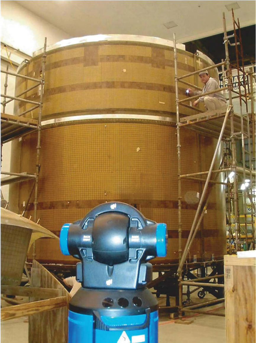
Figure 7-6. Use of laser technology for alignment of the assembly. (Courtesy NASA)
