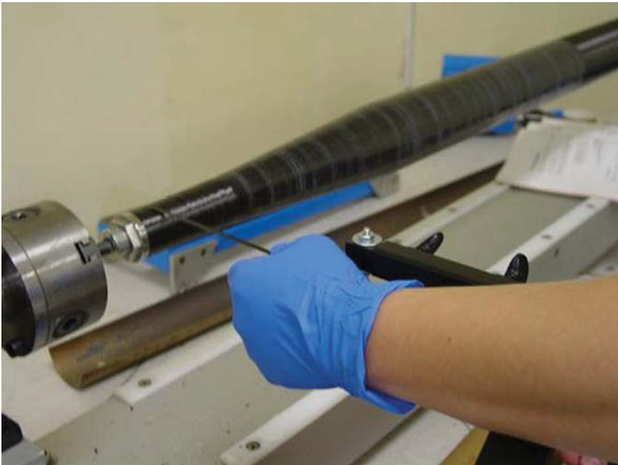
Figure 5-3. Paraplast ® mandrel mounted in the lathe and in the process of being wound. (Courtesy NASA)
