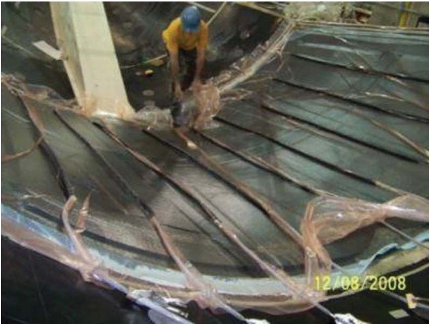
Figure 5-2. Resin infusion and bagging for a quarter-panel using the VARTM process.
