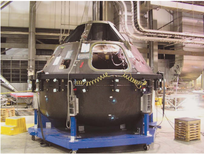
Figure 3-1. Full-scale CCM primary structure with fiber optic and traditional strain gages attached. (Courtesy NASA)
