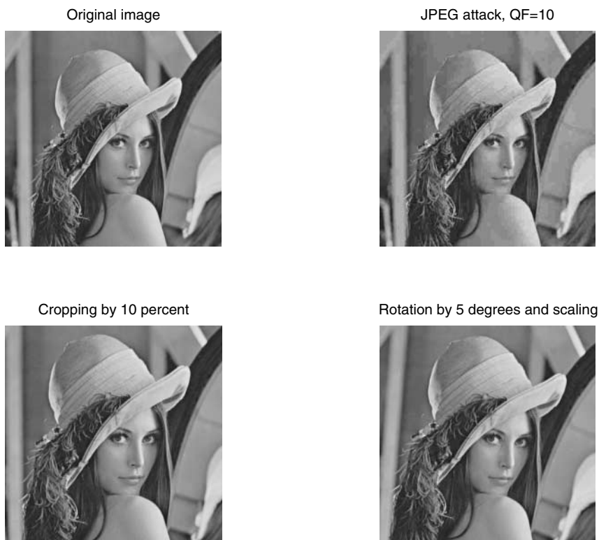
Fig. 1. Top left: original image Lena, top right: attacked version by JPEG compression with quality factor 10, bottom left: attacked version by cropping by 10 percent, bottom right: attacked version by rotation by 5 degrees and scaling
