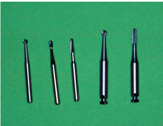
Fig. 26.8 A selection of tungsten-carbide burs. From the left: round, pear-shaped and tapered fissure high-speed handpiece burs. Round and crosscutting straight fissure burs for the slow-speed handpiece are shown on the right.
