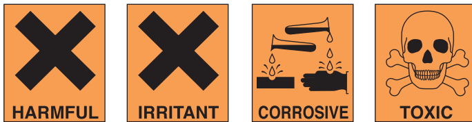
Fig. 3.1 Some common hazard warning signs
