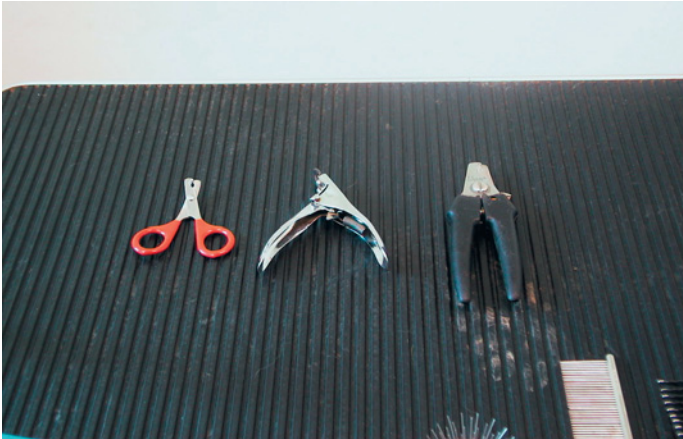
Fig 9.6 Nail clippers. Left to right: nail scissors, guillotine clipper, heavy duty pliers-type nail clipper
