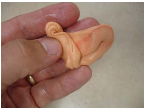
Fig. 10.4 Continued mixing of the compound and curing agent in hand for approximately 20 s
