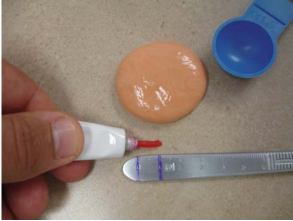
Fig. 10.2 Combine silicon compound with 1 cm of curing agent per one scoop (1 TSP) of compound. For a softer device, add slightly less curing agent. For a more firm device, add slightly more curing agent
