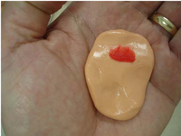
Fig. 10.3 Mix the compound and curing agent
