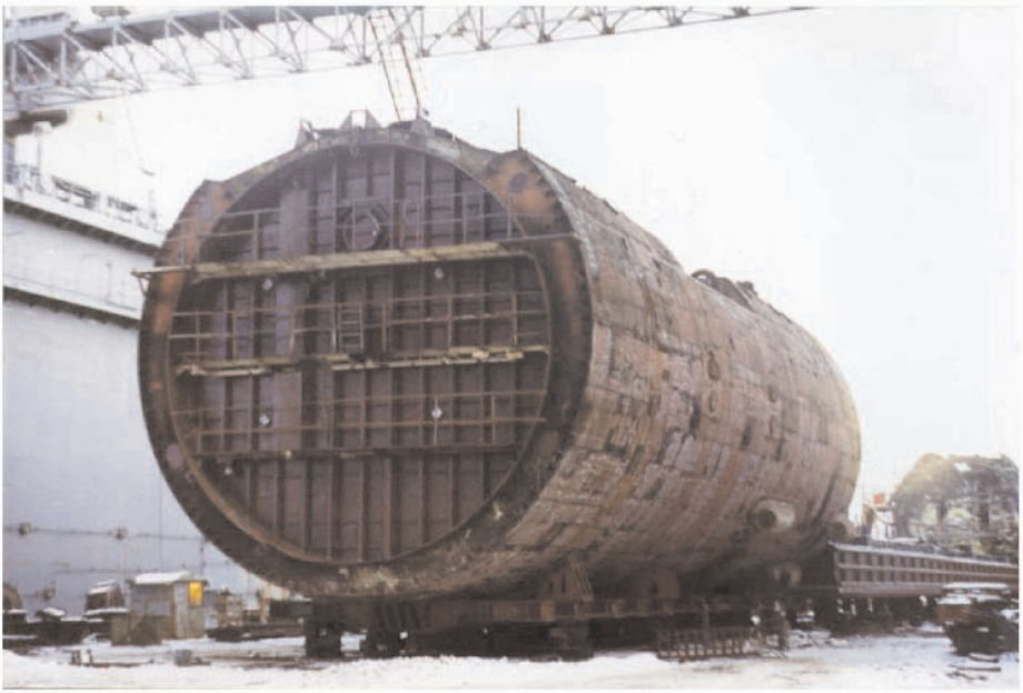
Figure 7. Three-compartment RC unit of NS dismantled on slip
