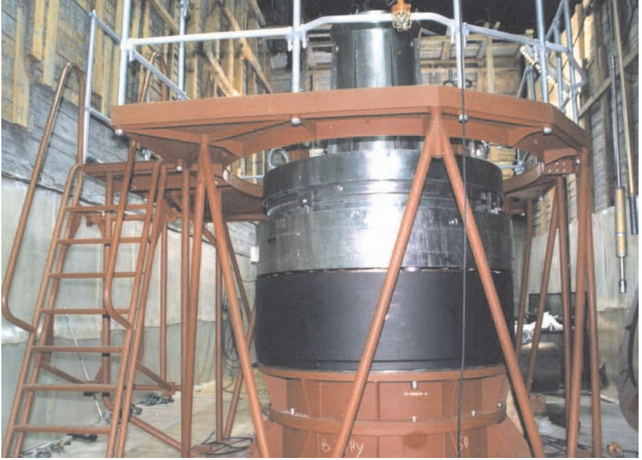
Figure 5. Full-scale test bench to check guiding mechanisms and containers
