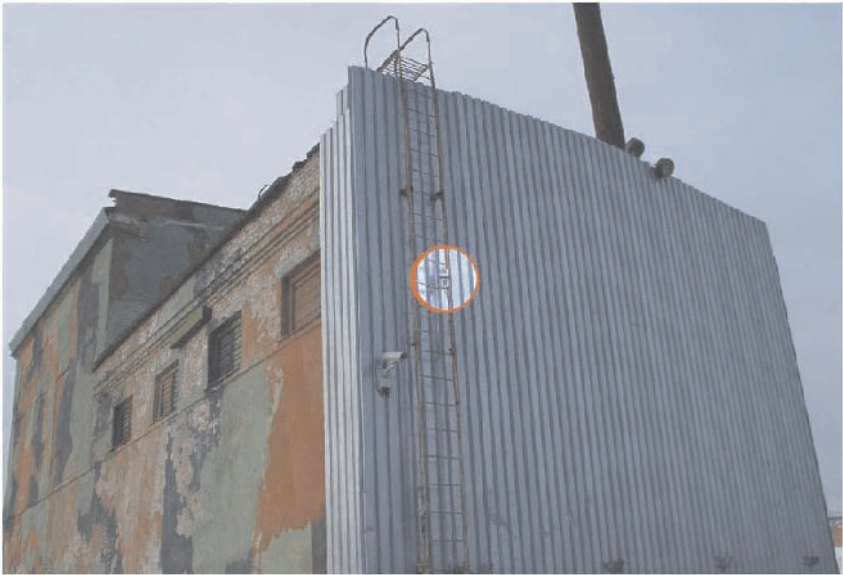
Figure 4. Exposure dose rate sensor at the process area of DalRAO (coastal maintenance base in Sysoeva Bay)
