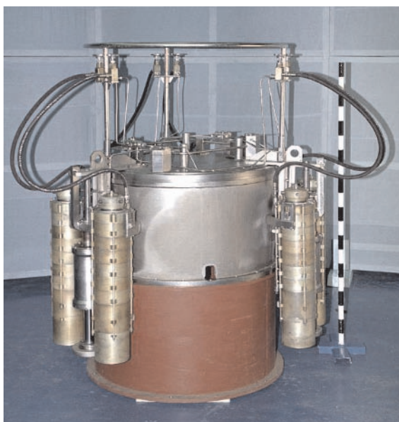
Figure 9. Device to turn/unscrew the screws on main connector
