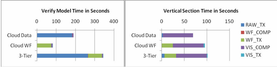
Fig. 6. Time profile comparison of a workflow with WF\_RATIO < 1 on the left and WF\_RATIO > 1 on the right. When WF\_RATIO < 1 , the preferred (non-local) strategy is to push the computation to the data using the Cloud WF configuration. When WF\_RATIO > 1 , the better strategy is to bring the data to the computation using the Cloud Data configuration.
