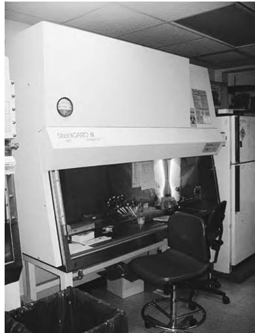
■ Figure 16-15 Laminar flow hoods are used to protect against biological hazards and to help maintain a sterile environment.
