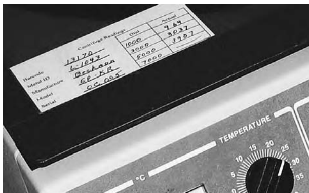
■ Figure 16-12 Centrifuge speeds are checked at least annually, and the results of actual and set speeds are posted on the instrument.
