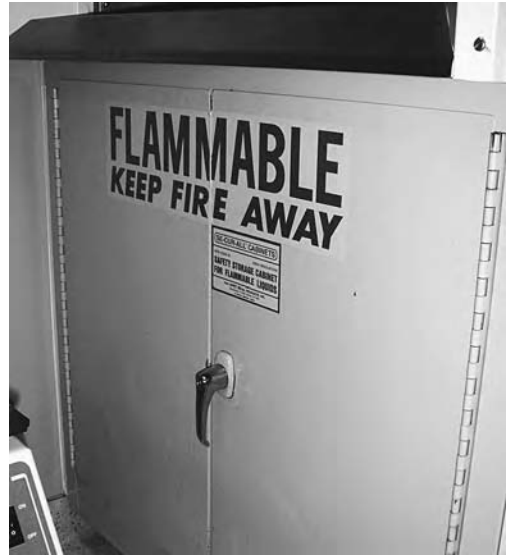
■ Figure 16-17 Flammable and explosive materials are stored in designated protective cabinets or explosion-proof refrigerators.
