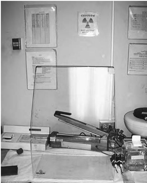
■ Figure 16-20 Acrylic shielding is required for working with gamma emitters, such as ^{32}\text{P} and ^{33}\text{P} .
