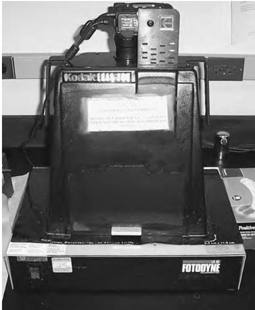
■ Figure 16-14 Cameras should be mounted securely for gel photography. A digital camera, shown here, is mounted on a photographic hood. A mask shields the ultraviolet light source except for the area where the gel is illuminated.
