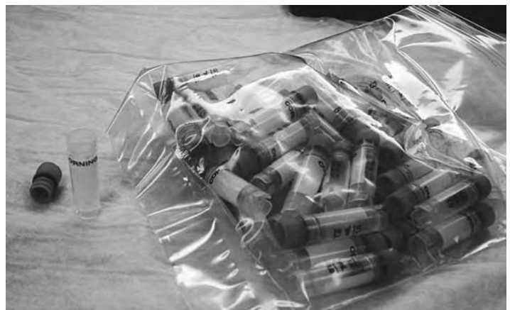
■ Figure 16-6 Cryotubes with tight-fitting lids are recommended for long-term freezer storage of DNA and RNA.
