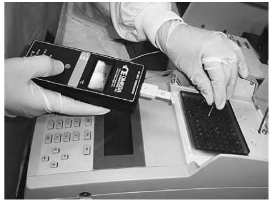
■ Figure 16-11 Block thermal cyclers may be monitored using a thermometer with a flexible probe. More thorough monitoring is performed with temperature probes and software that follows the ramping temperatures as well as the holding temperatures.
