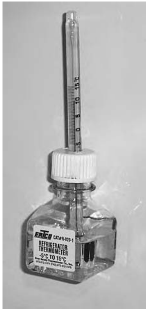
■ Figure 16-10 Certified chamber thermometers are used for monitoring temperatures in incubators, refrigerators, ovens, and freezers. The thermometers are supplied in plastic resin bottles containing liquid glycol.
