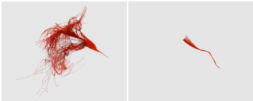
Fig. 1 Two different bunches emitted in two different locations from a source of size \sim \eta , recorded at time t = 75 \tau_\eta . On the left, a bunch emitted in a strong shear-rate region; on the right, a bunch emitted in a weak shear region. Direct Numerical Simulations are performed on a cubic fully periodic grid at 1024^3 points, at a Reynolds-Taylor number Re_\lambda \sim 300 . For further details see [30].
