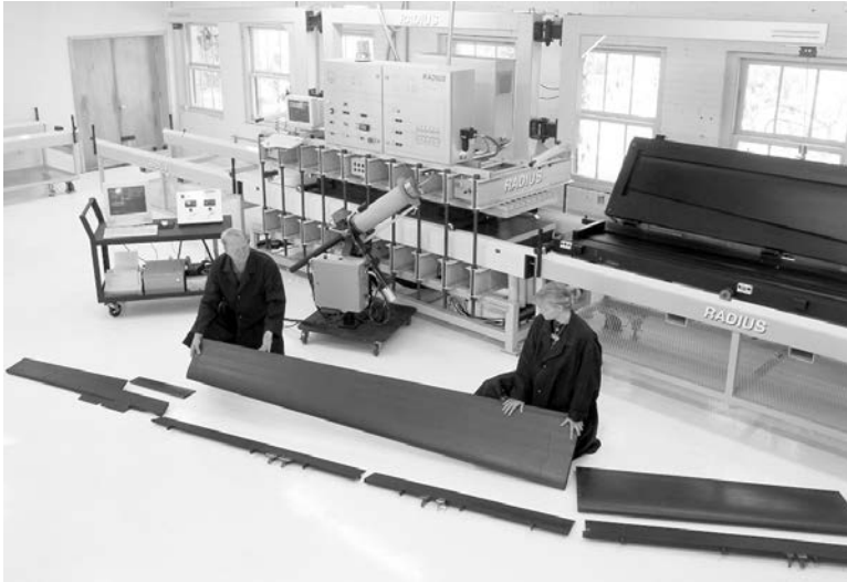
FIGURE 6.53 Outboard and inboard aircraft flaps, spoilers, and trim tabs. (Courtesy of Radius Engineering, Inc.)
