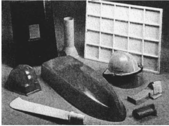
FIGURE 6.44 Typical small- to medium-sized resin transfer molded parts. (Courtesy of Liquid Control Corp.)
