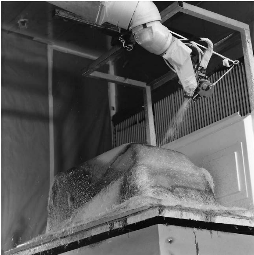
FIGURE 6.28 Robotic spray-up process for making a bathtub. The robot is applying chopped fiberglass with gel. (Courtesy of Fanuc Robotics.)
