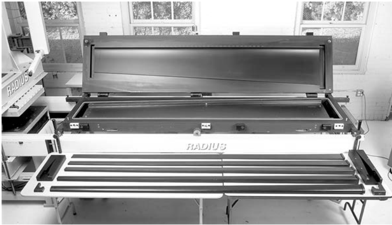
FIGURE 6.52 Molds and mandrels for making aircraft flaps. (Courtesy of Radius Engineering, Inc.)
