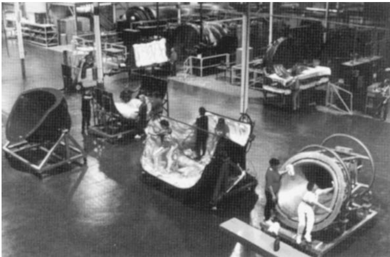
FIGURE 6.18 Manufacturing facility containing various autoclaves. (Courtesy of Marion Composites.)
