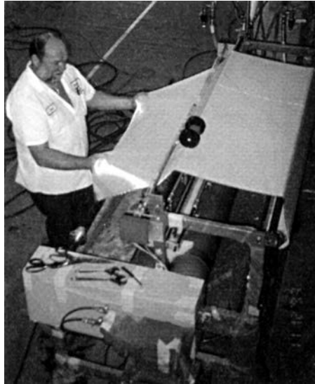
FIGURE 6.25 Fabric impregnator demonstrating impregnation of a glass fabric. (Courtesy of Merritt Boat and Engine Works, Pompano Beach, FL.)
