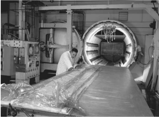
FIGURE 6.17 Vacuum bagged aerospace part ready to go inside an autoclave. (Courtesy of Lunn Industries.)
