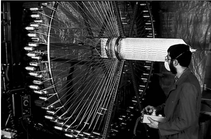
FIGURE 2.15 Braiding of fiberglass preform for an airfoil application. (Courtesy of Fiber Innovations Inc.)
