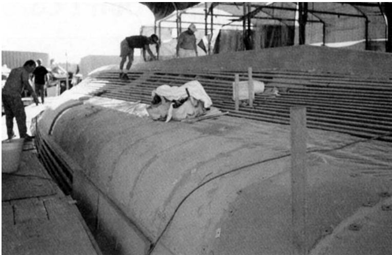
FIGURE 6.23 Crew members applying cross-linked foam core to a 72-ft yacht. (Courtesy of Mikelson Yachts, San Diego, CA.)
