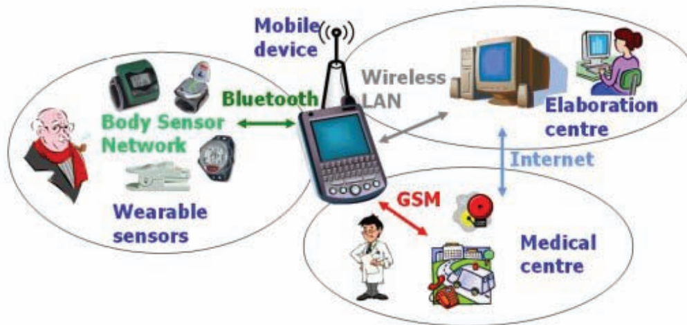
Figure 1. General architecture of a mobile health system
