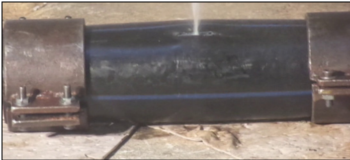
Fig. 5 Typical specimen failure of short-term burst tests
