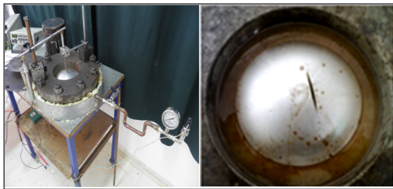
Fig. 2 Experimental setup for vapor bulging test
