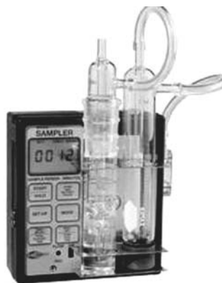
Figure 2.19 Impinger (liquid media) attached to a personal air sampling pump. (Courtesy of SKC, Inc., Eighty Four, PA.)
