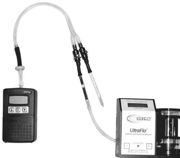
Figure 2.20 Orientation of dual sorbent tubes to sampling pump and calibration device. (Courtesy of SKC, Inc., Eighty Four, PA.)
