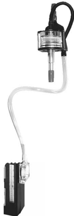
Figure 2.5 Cyclone adaptation for collection of respirable dust. (Courtesy of SKC, Inc., Eighty Four, PA.)
