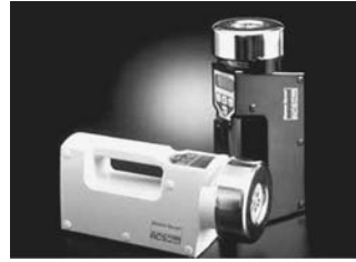
Figure 2.9 Two versions of the RCS are available; the newer version has digital air flow program capability.
