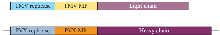
Figure 7.11 Schematic representation of a portion of the viral vectors used to produce full-size IgG antibodies in plants. In each case, the viral replicase and movement protein (MP) are cloned together with the gene (cDNA) for either a light chain or a heavy chain. The expression of each antibody gene is controlled by a promoter, a signal peptide (to ensure secretion), and a transcription termination region from the appropriate virus, none of which are shown. The viruses used included tobacco mosaic virus (TMV) and potato virus X (PVX). In both cases, the viruses were unable to replicate because of the absence of the viral coat protein. Recombinant viruses were introduced into plants as part of the T-DNA that is transferred during A. tumefaciens infection. doi:10.1128/9781555818890.ch7.f7.11
