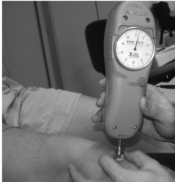
FIGURE 21.1 (See color insert.) Mechanical force transducer used to measure the force applied to the residual limb in the indentation test.
