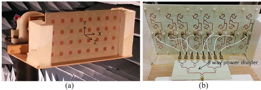
Fig. 5.14 Fabricated 4×8 dual-fed stacked-patch-antenna array. (a) Isometric view. (b) Back view
