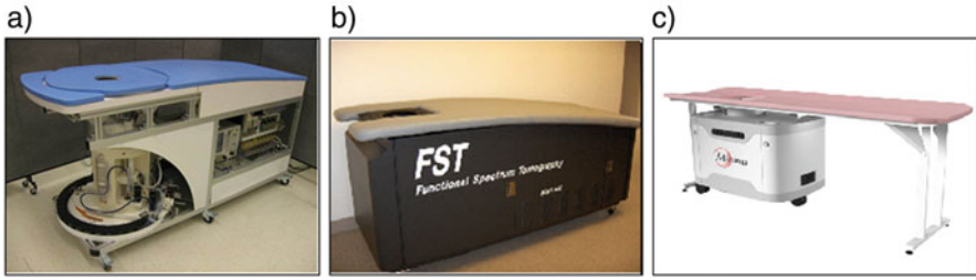
Fig. 16.10 Three examples of advanced microwave systems used for clinical assessment of breast imaging. (a) Monostatic radar with adaptive antenna positioning conforming to breast geometry (Courtesy University of Calgary) [81], (b) tomographic system equipped with circular arrays mechanically translated (Courtesy Microwave Imaging Syst. Tech. Inc.) [70], (c) multi-static radar system MARIA TM , electronic scan, and mechanical rotation (Copyright © Micrima Ltd. 2016) [71]
