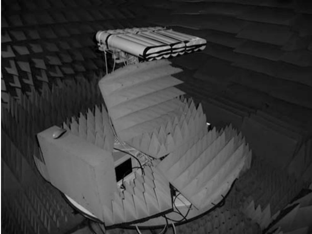
Fig. 4.20 Photo of the Yagi-Uda antenna array and its setup in the antenna range [6]
