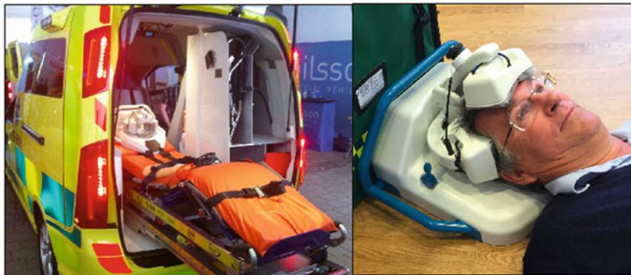
Fig. 16.12 Advanced microwave systems for brain stroke diagnostics based on classification technique (Courtesy Chalmers University, Medfield Diagnostics [99])
