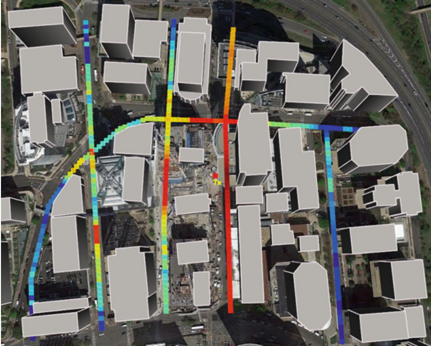
Fig. 12.5 The constructed 3D buildings of Rosslyn City, VA, using the method of Ref. [33] and the calculated path gains using ray tracing. The transmitter is located in the center of the image (The results are rendered in Google Earth)
