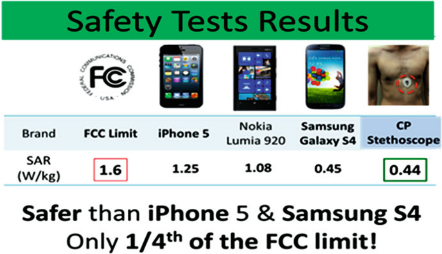
Fig. 2.26 Results from SAR measurements on the Cardio-Pulmonary Stethoscope
