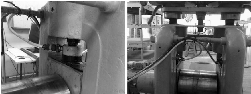
Fig. 7 Detail showing the location of tensometers on the rolling mill
