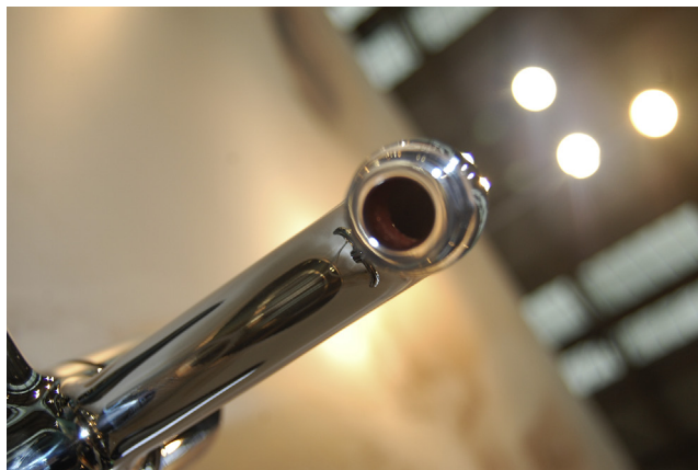
Figure 17.3 Smooth bore terminal flow straightener. This type of straightener is screwed into the tap outlet and is lined with alloys to reduce microbial contamination and biofilm growth.
