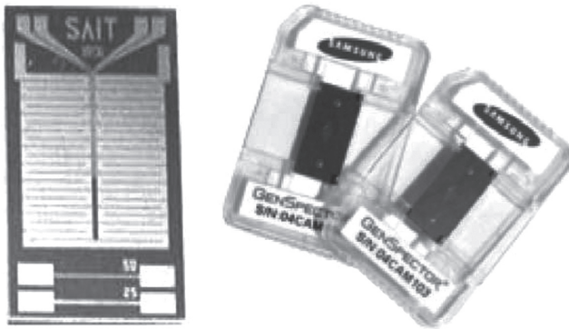
15.7 (a) Photograph of the rapid real-time microscale chip-based PCR system for screening of the hepatitis B virus infection. (b) The microfluidic PCR chip. (Source: Reprinted with permission from Cho et al. (2006), copyright 2006 Elsevier.)
