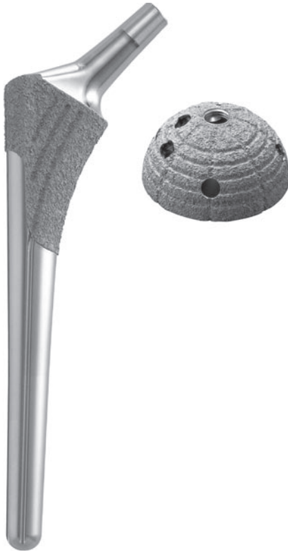
14.7 Stem and cup coated with hydroxyapatite using PROARC HA process, which is an inert-gas shield, arc-spray method originally developed by Japan Medical Materials Co. Ltd. Pure titanium is arc-sprayed to roughen the surfaces of stem and cup and then hydroxyapatite is flame-sprayed (with permission from Japan Medical Materials Corp.).
