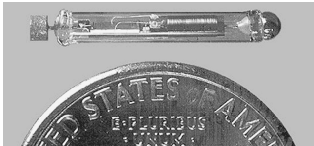
FIGURE 16.5 Microstimulator developed at A.E. Mann Foundation. Dimensions are roughly 2 \times 16 mm. Electrodes at the ends are made of tantalum and iridium, respectively.
