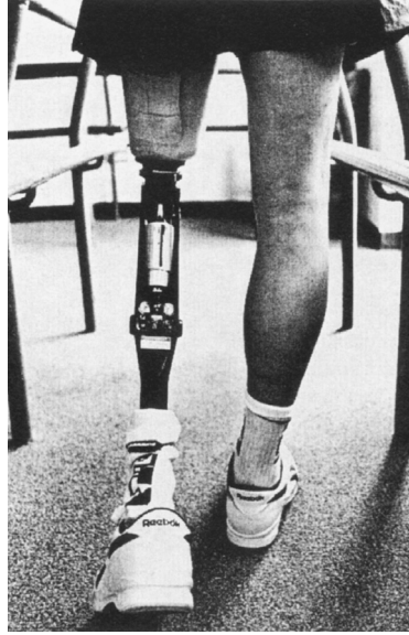
FIGURE 44.9 Endolite intelligent prosthesis in use, minus its cosmetic covers.
