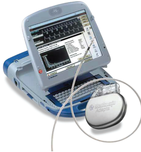
FIGURE 11.1 A pacing system comprises a programmer, pulse generator, and lead.
