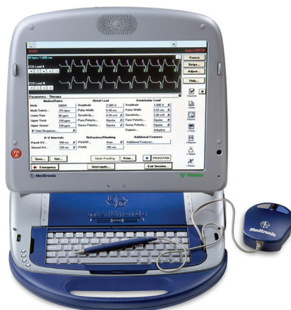
FIGURE 15.5 Programmer with transmitter/receiver unit that is placed in the vicinity of the implanted ICD. Long-range telemetry now eliminates the need for the transmitter/receiver in many ICD systems. (Reproduced with permission of Medtronic, Inc.)
