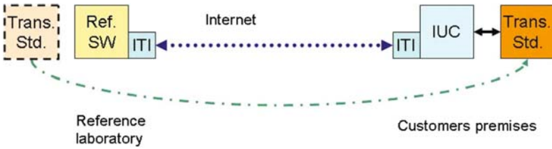
Fig. 6. Internet-supported calibrations with travelling reference standard. ITI: IT Interface, Trans. Std: Travelling reference standard, IUC: Instrument under calibration (in customer’s laboratory), Ref. SW: Reference laboratory’s software.
