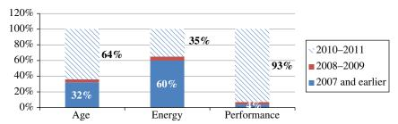
**FIGURE 21.9** In a recent server census in a Fortune 100 company's data center, 32% of the servers that were more than 4 years old consumed 60% of the energy while only producing 4% of the computing output performance. Courtesy of Intel Corporation.
