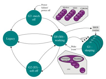
**FIGURE 21.10** ACPI power states and relationship among platform states, including Global (G-states), Sleep (S-states), microprocessor Performance (P-states), CPU (C-States), and Device (D-States). Courtesy of ACPI/Intel Corporation.
