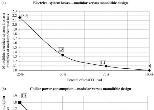
Monolithic chiller power as a multiplier of modular chiller power 1.7 1.6 1.5 1.4 1.3 1.2 1.1 1.0 1.0 1.0 50% 75% 25% 100% Percent of total IT load
