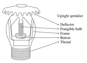
FIGURE 12.2 Standard upright sprinkler.
