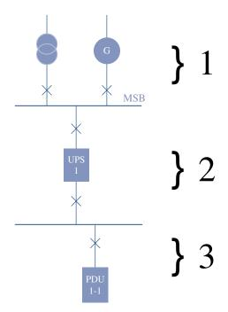
FIGURE 11.14 Power chain schematic.
