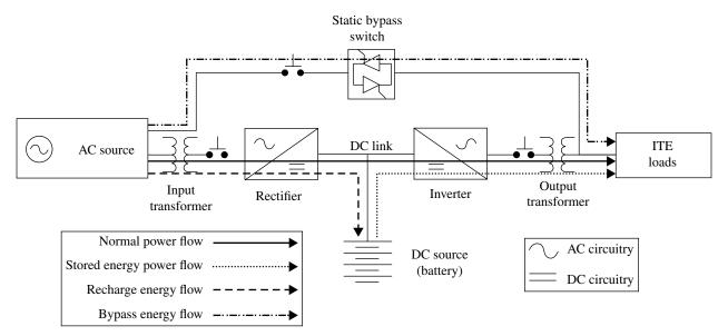
FIGURE 27.5 Typical transformer-based double-conversion UPS system. Courtesy of Eaton.
