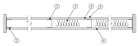
FIGURE 12.1 UL Design U465. Courtesy: Underwriters Laboratories. Reprinted from the Online Certifications Directory with permission from UL. © 2012 UL LLC.
