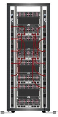
**FIGURE 29.11** Multiple power supply configuration. Courtesy of Raritan.
