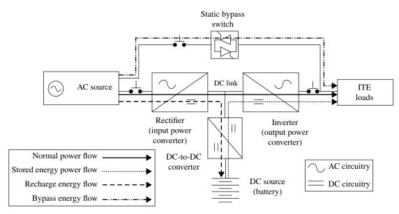
FIGURE 27.7 Basic transformerless double-conversion UPS power flow drawing. Courtesy of Eaton.
