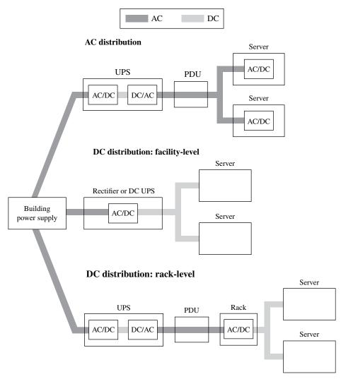
FIGURE 28.4 Data center power distribution systems [7].
