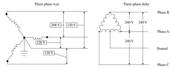
FIGURE 29.2 Three-phase wiring diagram. Courtesy of Raritan.
