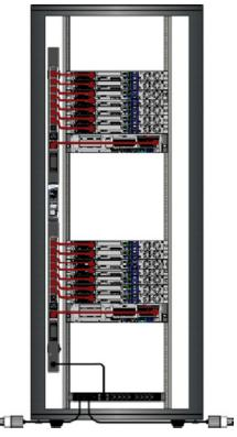
**FIGURE 29.9** Dual feed to single rack PDU with transfer switch. Courtesy of Raritan.
