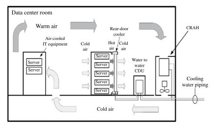
FIGURE 26.5 Side view: Rear-door cooling installation.
