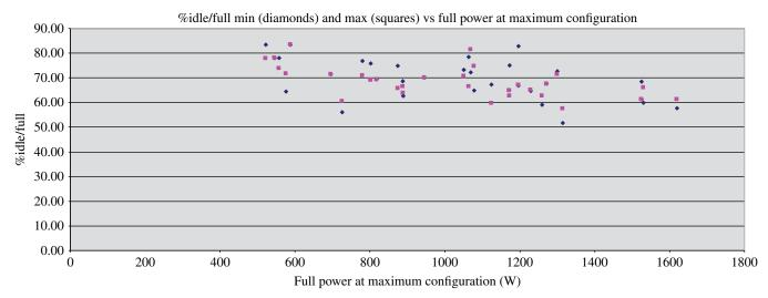
FIGURE 22.3 Idle power vs. full power for maximum configurations of Four processor socket server models. Courtesy of IBM.
