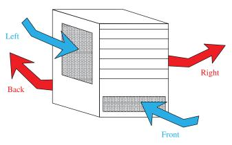
**FIGURE 9.1** Network chassis with front-to-back and left-to-right airflow (e.g., HP12504 model). Courtesy of Isaak Technologies Inc.
