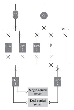
FIGURE 11.2 Parallel UPS redundant configuration.
