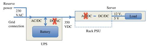
**FIGURE 28.2** Schematic sketch of a data center powered with DC. The conversions marked with crosses are removed with this alternative design. Note: 230 VAC from the power grid is the standard in Sweden.
