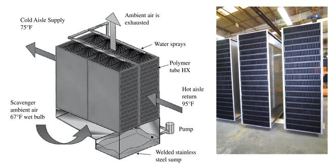
FIGURE 25.9 Integral heat exchanger/cooling tower or IECX.
