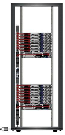
FIGURE 29.8 Single feed to single rack PDU. Courtesy of Raritan.
