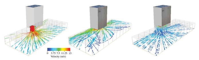
**FIGURE 17.10** Typical flow patterns—centrifugal blowers (left) and radial blowers (center and right). Courtesy of Future Facilities. Please visit companion website to access the color version of this figure.
