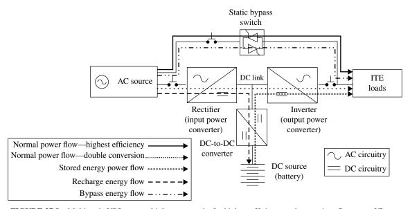
FIGURE 27.8 Multimode UPS uses multiple power paths for highest efficiency and protection. Courtesy of Eaton.
