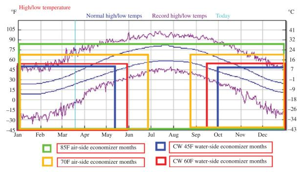
FIGURE 24.16 Appleton, Wisconsin, temperatures and economizer months. Courtesy of Weather Underground.
