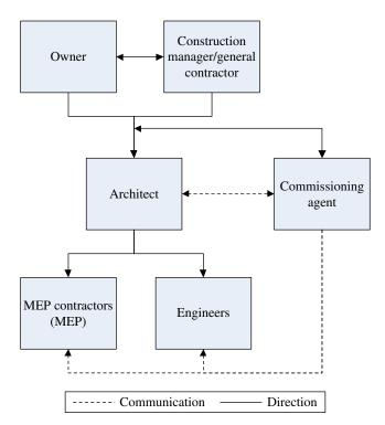
FIGURE 19.3 Lines of communication design/build.
