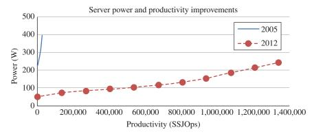
**FIGURE 21.2** Productivity has increased and energy use decreased significantly from 2005 to 2012. The SPECpower metric compares server performance at idle and every 10% utilization increase. Courtesy of Intel Corporation.
