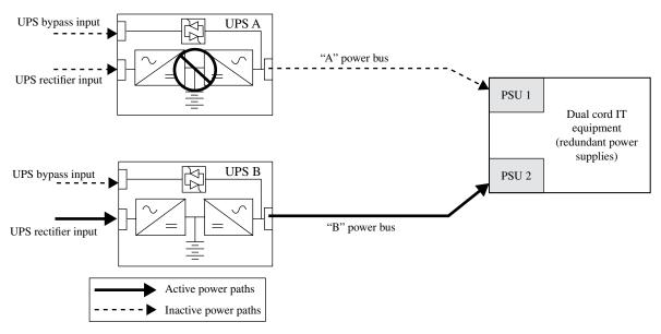
**FIGURE 27.20** Failure of one of the power paths or UPS forces the other UPS to assume the entire load; therefore, designs like this should be sized properly and continually monitored to reduce the chance of a UPS or power distribution system overload. Courtesy of Eaton.
