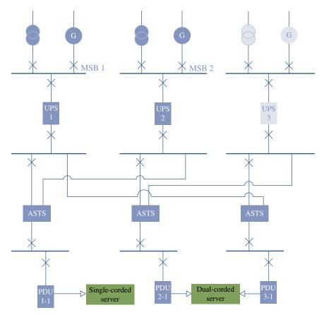
FIGURE 11.4 Distributed redundant configuration.
