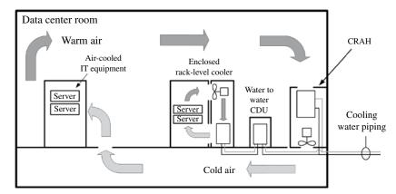
FIGURE 26.3 Side view: Enclosed rack-level cooler installation.
