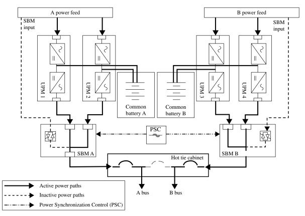
**FIGURE 27.25** The hot tie cabinet (HTC) allows concurrent maintenance of the upstream A or B bus while the downstream loads stay powered by both buses. Courtesy of Eaton.
