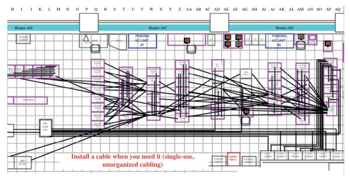
FIGURE 14.1 Example of computer room with unstructured nonstandard cabling.
