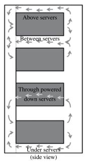
**FIGURE 17.13** Schematic of internal cabinet recirculation. Courtesy of Future Facilities.
