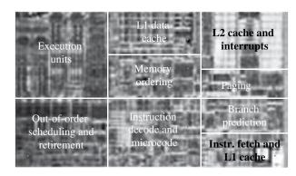
**FIGURE 21.4** Photograph of a single core in the Intel® Xeon® processor E5-26xx series die, annotated with the major function blocks (one single core rotated 90° from Figure 21.3). Courtesy of Intel Corporation.
