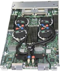
FIGURE 26.9 Water-cooled servers. Courtesy of IBM Corporation and Asetek Inc.
