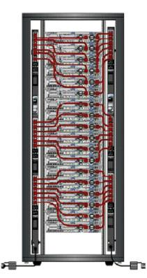
FIGURE 29.10 Dual feed to dual rack PDUs. Courtesy of Raritan.
