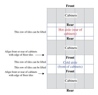
FIGURE 14.11 Cabinet placement example.
