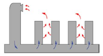
**FIGURE 24.5** Flooded return—fully ducted supply. Courtesy of Schneider Electric.
