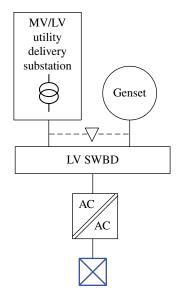
FIGURE 15.16 Single-line diagram of the MV/LV power system.
