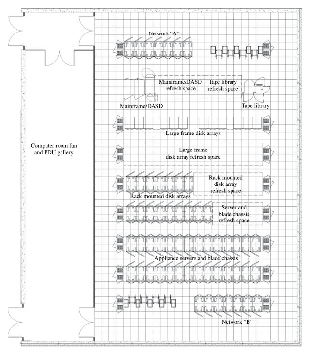
FIGURE 9.6 Example of multiplatform computer room with 18% space required for technology refresh. Courtesy of Isaak Technologies.
