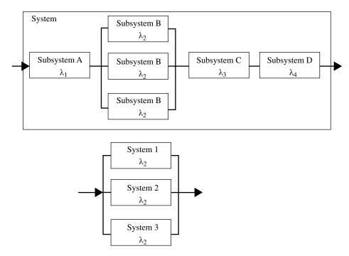
FIGURE 27.13 Upper drawing shows subsystem redundancy, while lower drawing shows parallel redundancy. Courtesy of Eaton.
