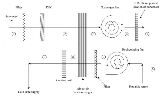
**FIGURE 25.5** Schematic of typical indirect air-side economizer.
