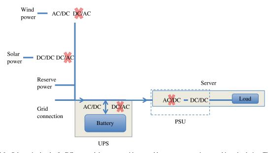
**FIGURE 28.6** Schematic sketch of a DC-powered data center with renewable energy sources integrated into the design. The conversions marked with crosses are removed with this alternative design.
