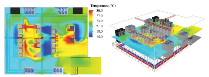
**FIGURE 17.6** Result plane of temperature and halfway cabinet. Courtesy of Future Facilities. Please visit companion website to access the color version of this figure.
