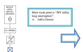
Unexpected event : "load loss" Failure frequency Unavailability Failures/year Hours/year 0.89 3.27
