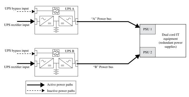
**FIGURE 27.19** Typical dual-bus power system with separate UPS systems feeding the different power distribution buses. This type of deployment puts the power failure point at the individual IT device, ensuring the highest levels of availability. Courtesy of Eaton.
