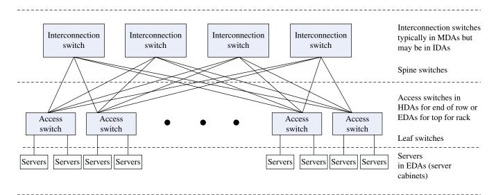
**FIGURE 14.12** Data center switch fabric example.
