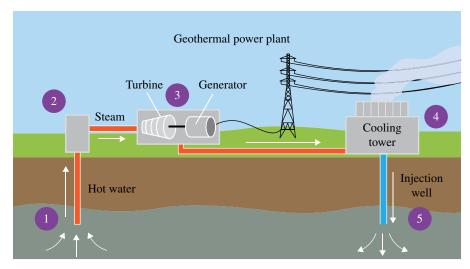
FIGURE 30.11 Diagram of a geothermal power plant. From www.epa.gov.
