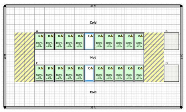
FIGURE 24.12 Hot aisle containment system configuration. Courtesy of Schneider Electric.
