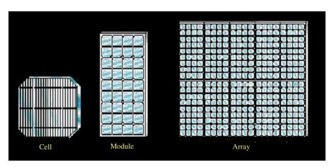
**FIGURE 30.4** PV cells, modules, and arrays. Photo illustration from the U.S. Department of Energy, Energy Efficiency, and Renewable Energy Program.
