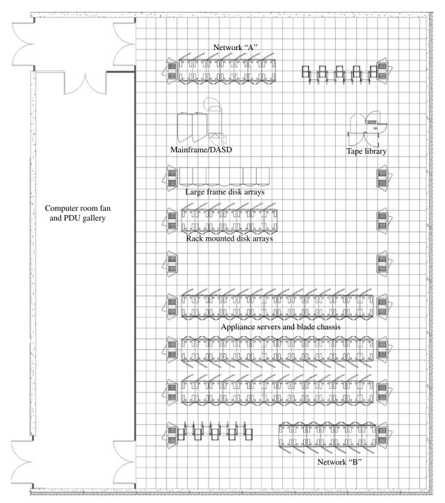
FIGURE 9.5 Example of multiplatform computer room layout. Courtesy of Isaak Technologies.
