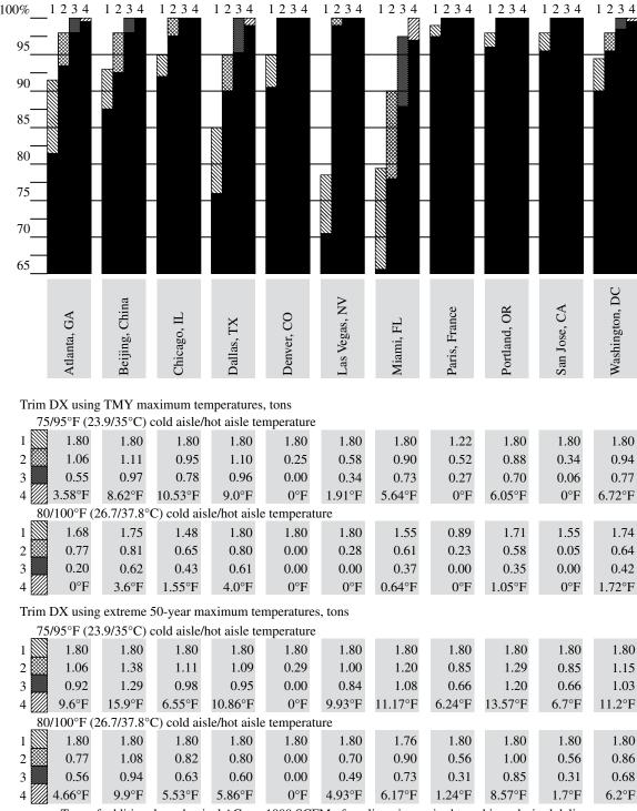
Tons of additional mechanical AC per 1000 SCFM of cooling air required to achieve desired delivery temperature when using air economizers—with no economizer, the full AC load is 1.8 tons/1000 SCFM.
