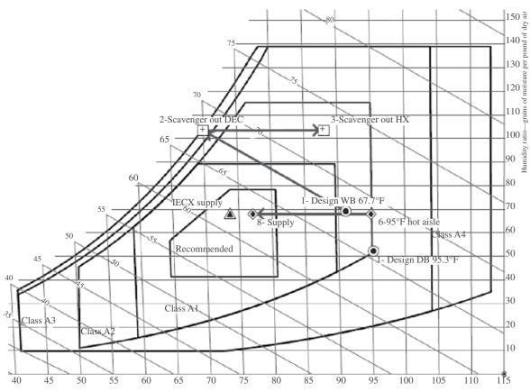
**FIGURE 25.6** Psychrometric chart showing recommended and allowable envelopes of temperature and moisture content of delivered cooling air for datacom facilities.
