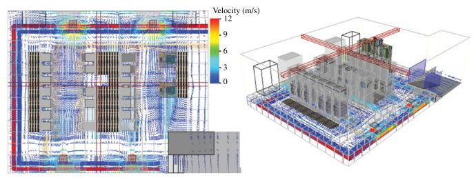
**FIGURE 17.7** Result plane of flow pattern in a floor void. Courtesy of Future Facilities. Please visit companion website to access the color version of this figure.
