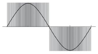
**FIGURE 27.1** PWM switching pattern is filtered into clean sine wave AC output waveform. Courtesy of Eaton.
