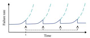
Periodical maintenance permits to guarantee constant equipment failure rate.
