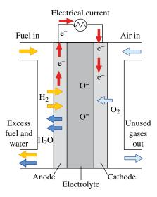
**FIGURE 30.17** Solid oxide fuel cell. Photo courtesy of EERE, Department of Energy.
