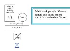
Unexpected event : "load loss" Failure frequency Unavailability
