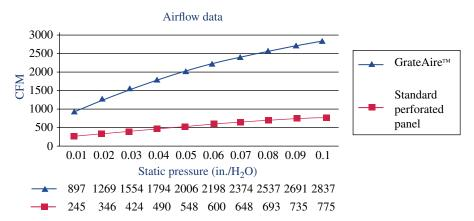
FIGURE 23.4 Performance of perforated tiles and grates. (Data from Tate Access Floors.)
