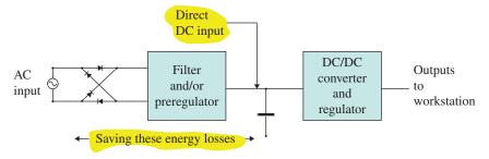
FIGURE 28.3 Schematic sketch showing which conversions can be eliminated in the DC PSU compared to the AC solution.
