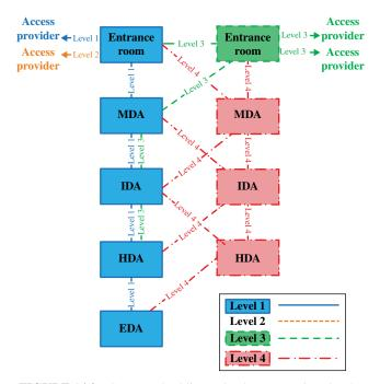
FIGURE 14.9 Structured cabling redundancy at various levels.
