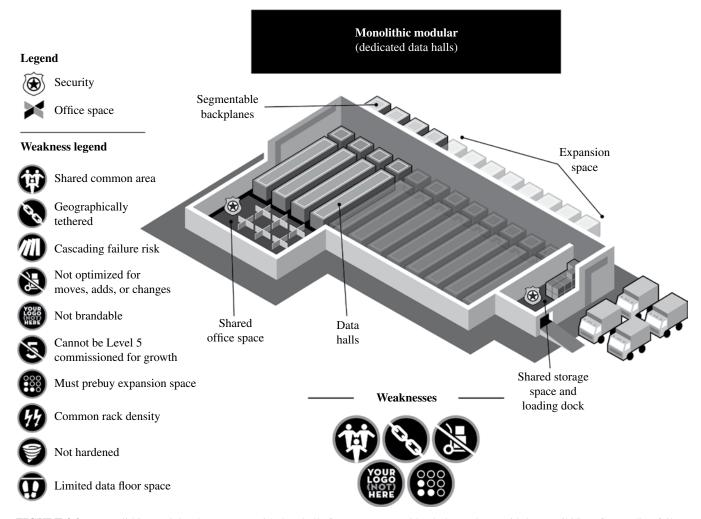
**FIGURE 3.2** Monolithic Modular data centers with data halls feature segmental backplanes that avoid the possibility of cascading failure found with traditional designs. Courtesy of Compass Data Centers.
