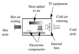
FIGURE 26.2 ICT equipment cooling basics.
