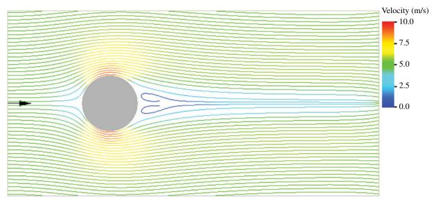
**FIGURE 17.8** Streamline flow around a cylinder. Courtesy of Future Facilities. Please visit companion website to access the color version of this figure.
