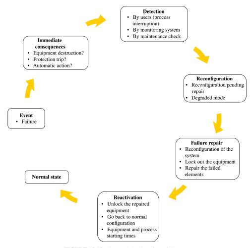
FIGURE 15.14 System behavior after a failure.
