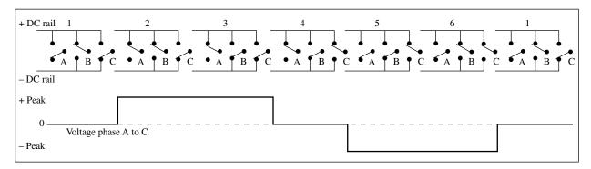
**FIGURE 27.6** The six-step inverter switching sequence and voltage waveform for a three-phase UPS. The voltage waveform is for phases A to C of the inverter output. Courtesy of Eaton.
