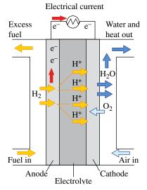
**FIGURE 30.13** Diagram of PEM fuel cell. Photo courtesy of EERE, Department of Energy.
