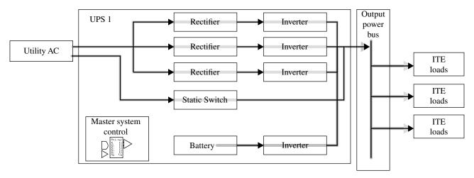
FIGURE 27.12 Single UPS system with some internal redundancy provided for rectifier and inverter. Courtesy of Eaton.
