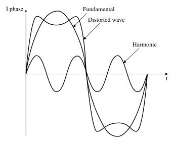
FIGURE 28.5 Example of electrical harmonics.
