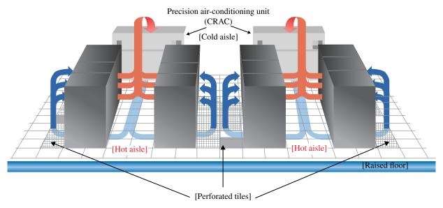
**FIGURE 24.1** Hot aisle/cold aisle configurations with raised floor. Courtesy of Emerson Electric Corp.
