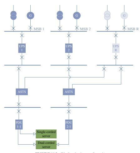
FIGURE 11.3 Block redundant configuration.
