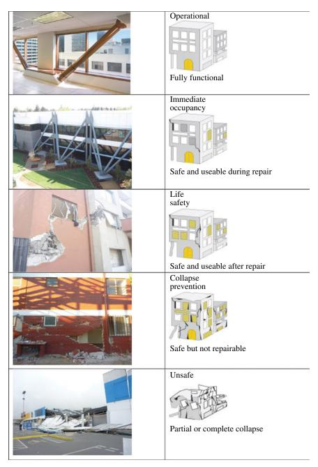
FIGURE 13.1 Building performance states. Courtesy and © Degenkolb Engineers, 2013.
