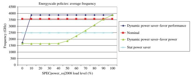
FIGURE 22.2 Processor power management function. Courtesy of IBM.
