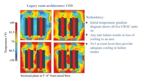
FIGURE 24.15 Legacy room cooling redundancy check CFD. Courtesy of Schneider Electric.
