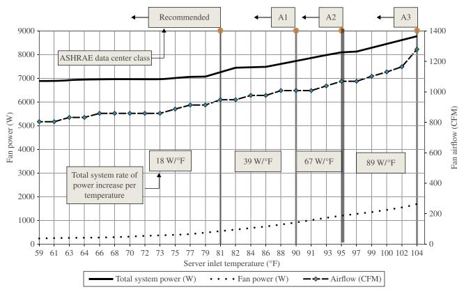
**FIGURE 2.15** Increasing supply air temperature to the server by moving from ASHRAE environmental class "Recommended" to "A3" will increase not only server airflow but also the rate of change of power increase per °F. Finding the right balance point of cooling system energy efficiency and server energy use must happen on a case-by-case basis.
