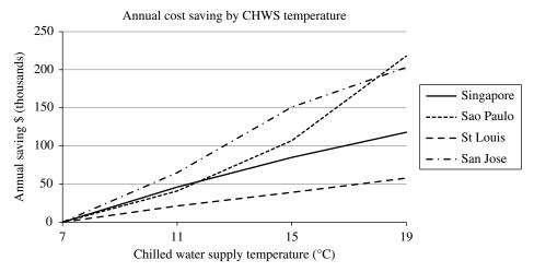
**FIGURE 6.8** Energy cost sensitivity analysis—annual cost saving by chilled water supply (CHWS) temperature.
