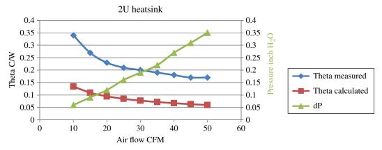
FIGURE 26.6 Heat sink characterization.
