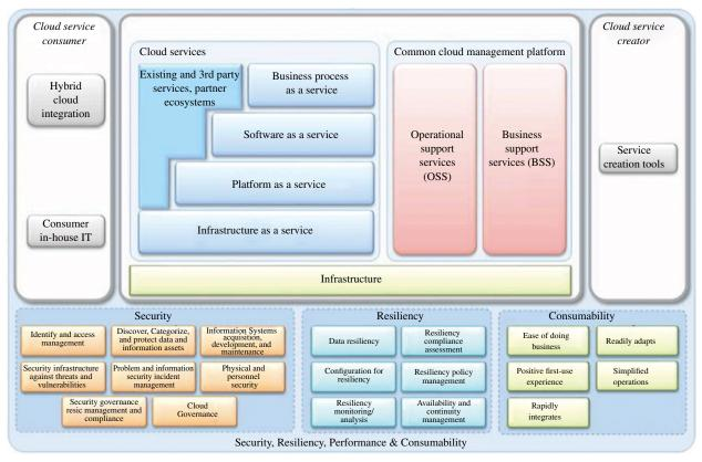
FIGURE 20.7 Cloud computing reference architecture (Courtesy of IBM Corporation).
