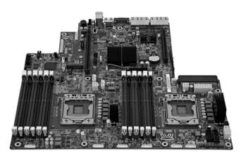
**FIGURE 21.7** Intel® Xeon® E5-2400 Server Motherboard. Airflow is designed for front to rear to minimize the parts in the heat shadow of the microprocessors and memory DIMMs. Courtesy of Intel Corporation.
