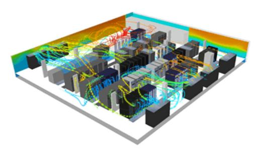
FIGURE 24.8 Room-based cooling system. Courtesy of Schneider Electric.
