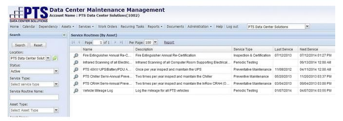
**FIGURE 34.4** Service routine details. Courtesy of PTS.
