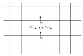
**FIGURE 17.2** Slice through mesh showing connectivity, values, and fluxes. Courtesy of Future Facilities.
