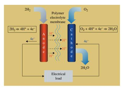
FIGURE 30.12 Block diagram of a fuel cell. Diagram from EPA, http://www.epa.gov/fuelcell/basicinfo.htm#background.
