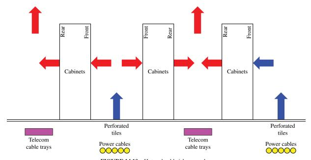
FIGURE 14.10 Hot and cold aisle examples.
