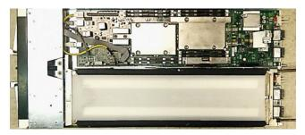
**FIGURE 26.11** Clustered systems' phase change-cooled blade with two half-width servers. Courtesy of Clustered Systems, Inc.
