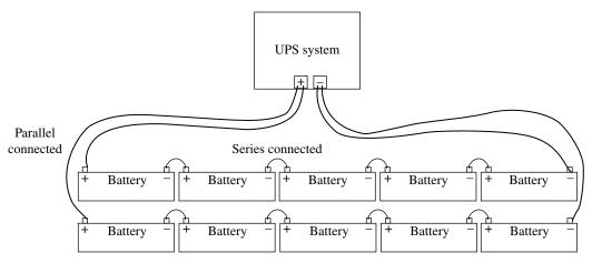
FIGURE 27.14 A way to increase UPS backup energy (DC) reliability is to parallel multiple battery strings. Courtesy of Eaton.
