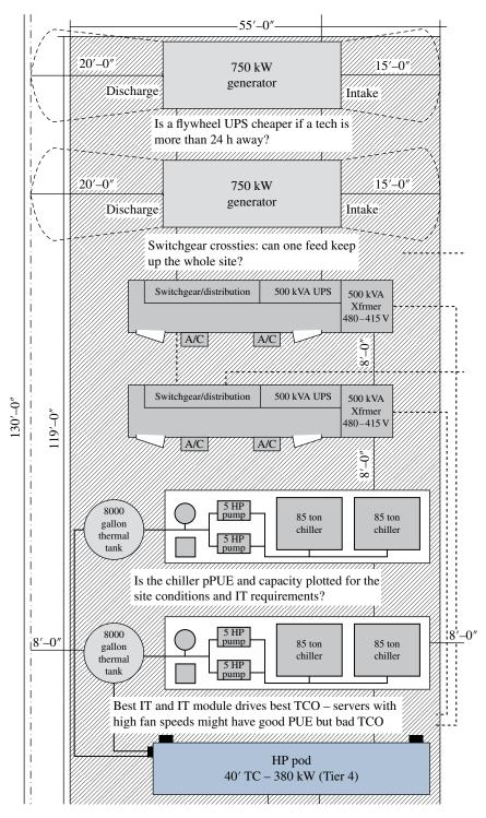
**FIGURE 4.18** An MDC can have parts from all sources, so make sure you know who is responsible for what. All IT work/rack, container pPUE, and chiller efficiencies are not equal, and the TCO is based on how much IT performance you get out of the whole solution, not just one of the parts. Courtesy of Hewlett-Packard Company.
