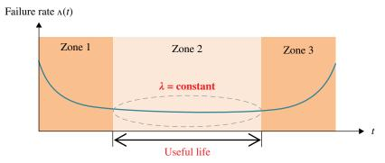
FIGURE 15.4 Failure rate curve.
