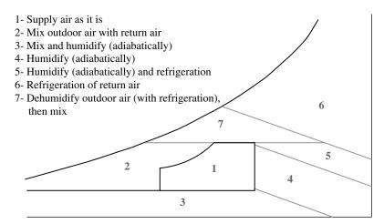
**FIGURE 4.9** Psychrometric chart showing how air must be conditioned to make it acceptable to a define IT entering state. HP CFS Whitepaper "Global Data Centre Energy Strategy" 10-18-2009, Courtesy of Hewlett-Packard Company.
