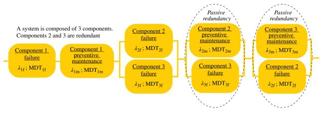
FIGURE 15.9 Reliability calculation of 2 redundant components taking into account preventative maintenance.
