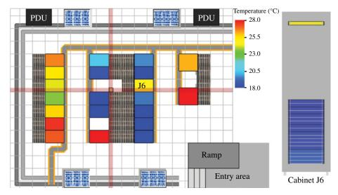
**FIGURE 17.14** Maximum inlet temperature—room plan view (left) and individual cabinet view (right). Courtesy of Future Facilities. Please visit companion website to access the color version of this figure.
