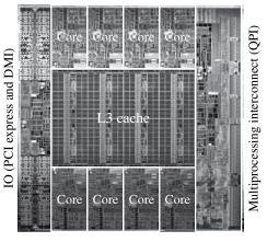
**FIGURE 21.3** Photograph of Intel® Xeon® processor E5-26xx series die. The picture has been annotated to show the various major functional blocks: Cores and Uncore (everything else, including Cache, IO, multiprocessing interconnect, etc.). Courtesy of Intel Corporation.
