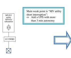
Unexpected event: "load loss" Failure frequency Unavailability Failures/year Hours/year 9.65 3.12
