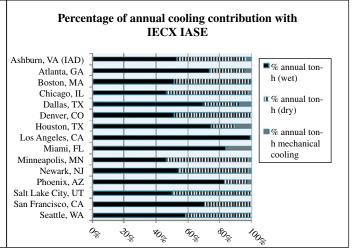
FIGURE 25.13 Analysis summary for modular data center cooling solution using IECX.
