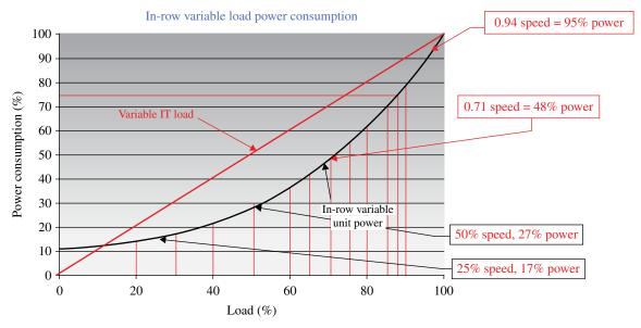
FIGURE 24.14 Fan power curve affinity law. Courtesy of Schneider Electric.
