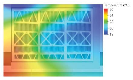
**FIGURE 17.9** Typical return air temperature variation at a down flow unit return. Courtesy of Future Facilities. Please visit companion website to access the color version of this figure.
