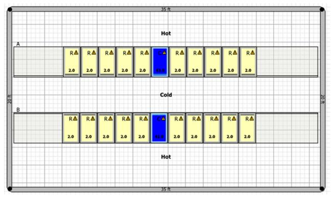
FIGURE 24.11 Cold aisle open system configuration. Courtesy of Schneider Electric.
