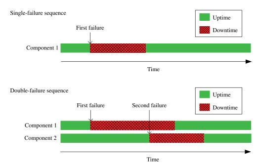
FIGURE 15.19 Single- and double-failure time sequence graphs.
