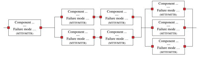
FIGURE 15.20 Reliability block diagram principle.
