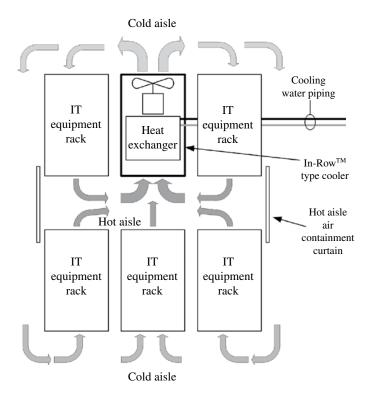
**FIGURE 26.4** Overhead view: In-Row<sup>TM</sup> rack-cooler installation.
