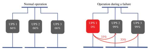
**FIGURE 11.6** N+1 normal operation and failure scenarios.
