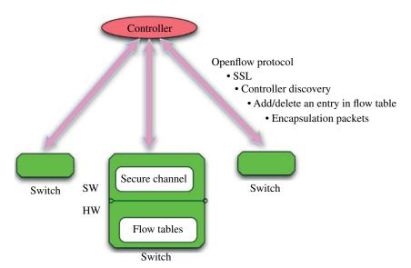
FIGURE 20.4 SDN controller approach.
