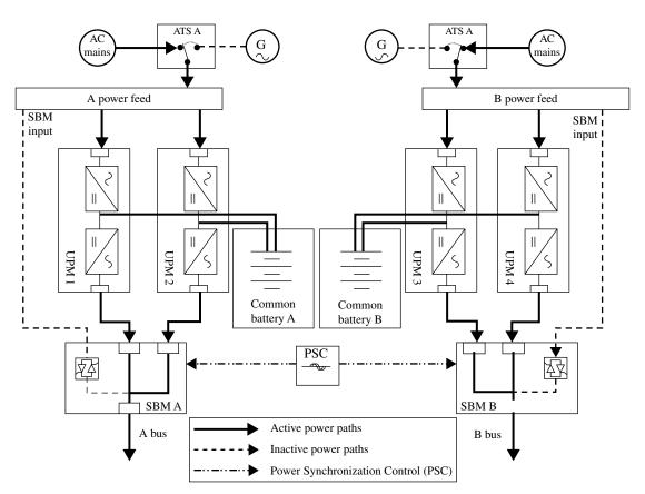
**FIGURE 27.24** Multiple N + 1 UPS systems can be used in a dual-bus configuration. Each bus has its own system bypass module (SBM), and upstream ATS with generator. A common battery is used for each group of uninterruptible power modules (UPM). Courtesy of Eaton.
