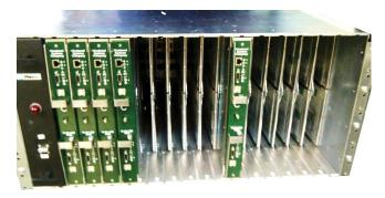
**FIGURE 26.12** Sixteen-blade chassis. Courtesy of Clustered Systems, Inc.
