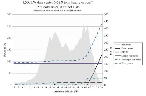
FIGURE 25.12 Power consumption for a typical IECX IASE cooling unit.
