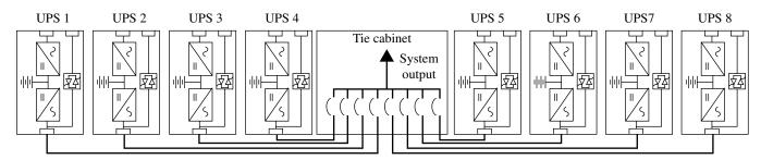
FIGURE 27.18 This distributed bypass configuration has eight UPS modules paralleled into a single system. Courtesy of Eaton.
