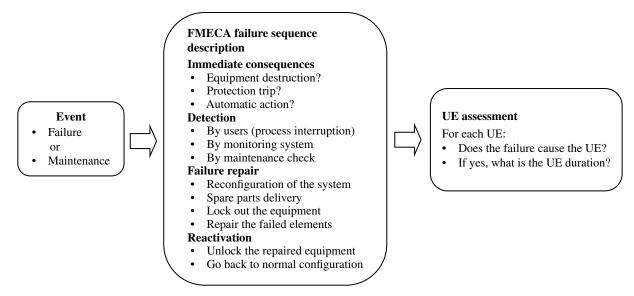
FIGURE 15.18 Assessment principle of an equipment failure mode during a FMECA approach.
