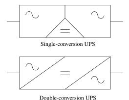
**FIGURE 27.4** IEEE accepted drawings for different static UPS designs. Courtesy of Eaton.
