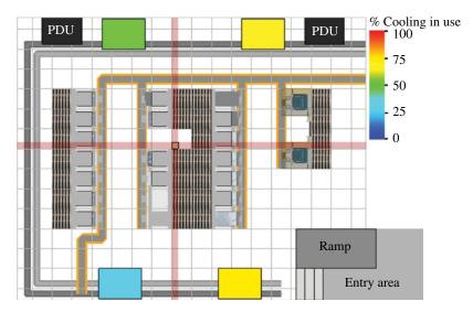
**FIGURE 17.16** Cooling unit load. Courtesy of Future Facilities. Please visit companion website to access the color version of this figure.
