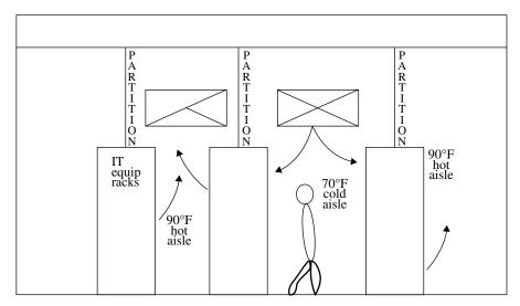
FIGURE 10.2 Hot aisle-cold aisle.
