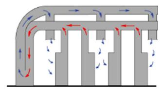
FIGURE 24.4 Fully ducted return—locally ducted supply (Left, Raised floor; Right, Overhead). Courtesy of Schneider Electric.
