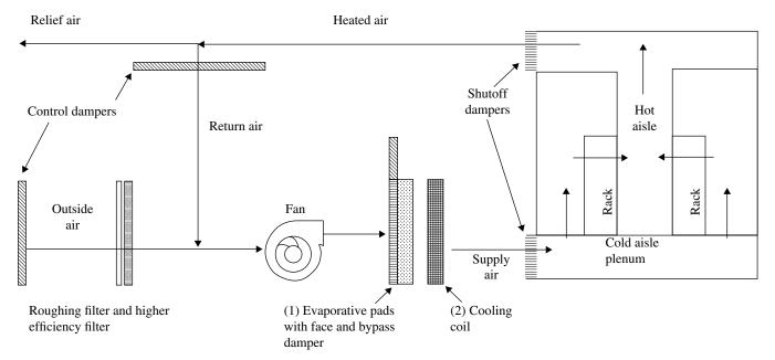
FIGURE 25.1 Schematic of a typical direct air-side economizer.
