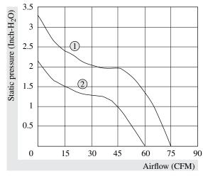
FIGURE 26.7 Fan curves 60 mm × 60 mm.
