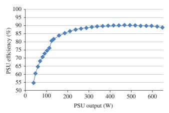
**FIGURE 21.6** Power Supply Efficiency depends on the amount of power it is delivering and usually decreases rapidly at lower power output levels. Courtesy of Intel Corporation.
