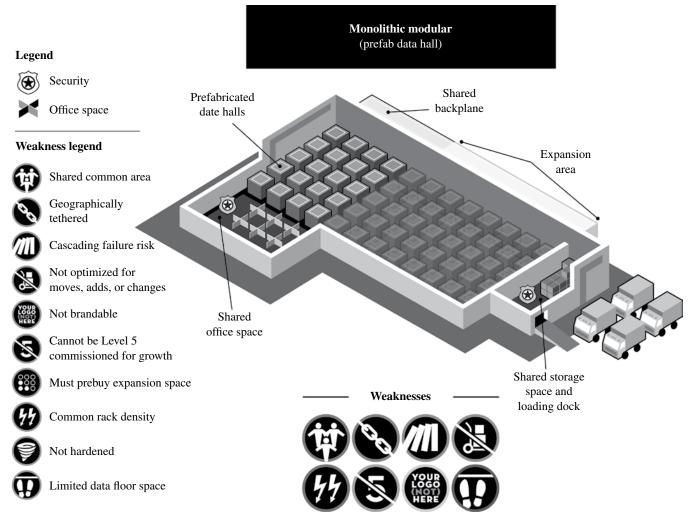
**FIGURE 3.4** Monolithic Modular data centers with prefabricated data halls use a shared backplane architecture that raises the risk of cascading failure in the event of an attached unit. Courtesy of Compass Data Centers.
