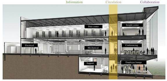
Cross section view into the ESIF HPC data center. Mustration from SmithGroupJJR
