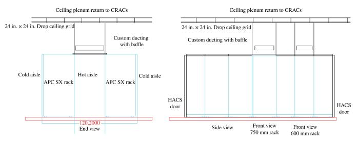
FIGURE 24.7 Baffle duct kits for HACS. Courtesy of Schneider Electric ITB.
