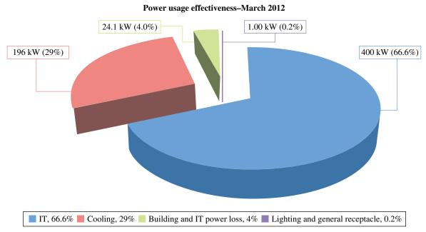
**FIGURE 1.1** The DOE national average PUE for data centers is 1.75. 50B-1275 data center has evolved from an average PUE of 1.65 (calculated in 2009) to today's 1.47. Getting there, staying there, and further improving the PUE is an ongoing effort (Source: Nina Lucido, Data Center Utilization Report, March 2012, LBNL, U.S. Department of Energy. https://commons.lbl.gov/display/itdivision/2012/04).
