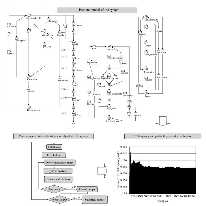
FIGURE 15.24 Time sequential stochastic simulation algorithm of a system.
