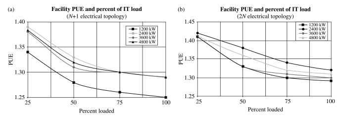
**FIGURE 2.5** (a) and (b) Electrical system topology and percent of total IT load will impact overall data center PUE. In this example, a scalable electrical system starting at 1200 kW and growing to 4800 kW is analyzed. The efficiencies vary by total electrical load as well as percent of installed IT load.
