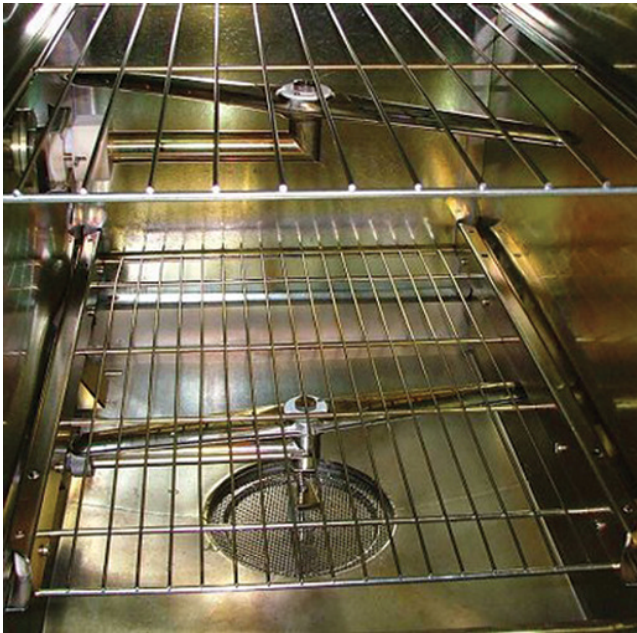
Figure 7.17 Scaling and staining of the interior walls and floor of a thermal washer disinfectator which has been connected to an unsuitable water supply; compare the sheen on the horizontal shelf to the staining of the other surfaces. Source: Courtesy of Paul Jenkins.
