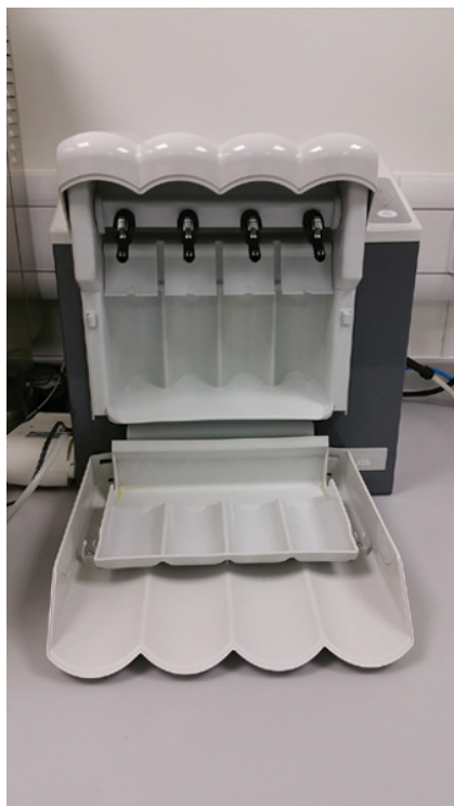
Figure 7.10 Dental handpiece cleaning and lubricating machine, which cleans up to four handpieces.
