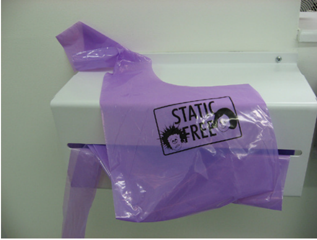
Figure 6.10 Antistatic disposable aprons in a wall-mounted dispenser.
