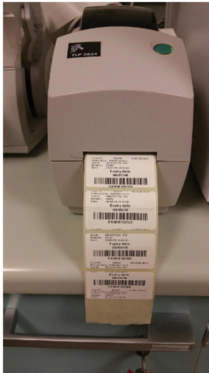
Figure 7.21 An example of an automated label printer linked to the sterilizer microprocessor.
