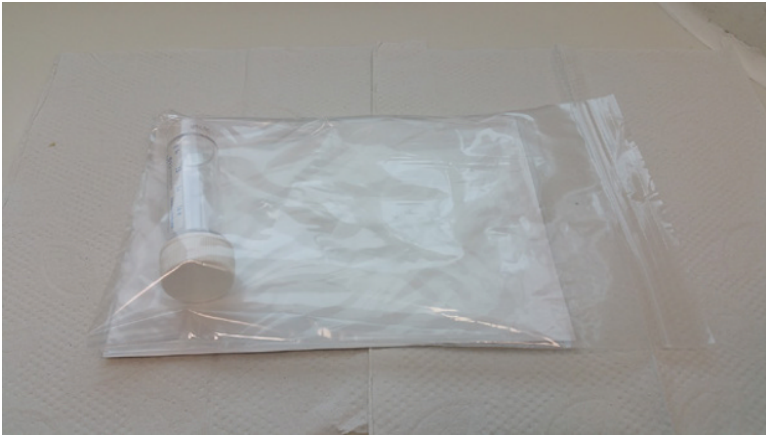
Figure 11.1 A specimen bottle (primary packaging) in a zip-lock self-sealing specimen bag (secondary packaging); note the separate outer pouch for placement of the request form.
