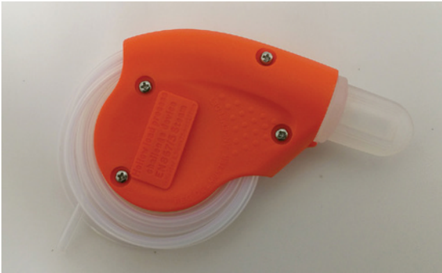
Figure 7.19 Helix test. If the vacuum pump is working correctly, air is withdrawn from the narrow-bore tubing and replaced with steam that penetrates to the indicator test strip, which will change colour.
