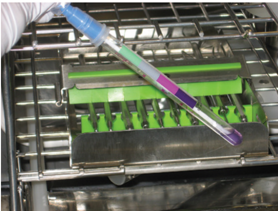
Figure 7.15 Protein detection test. (a) A random set of instruments and tray are swabbed and the swab is inserted into the test solution of ninhydrin. If protein is present the solution will turn blue-purple. (b) A pass test. (c) A fail.
