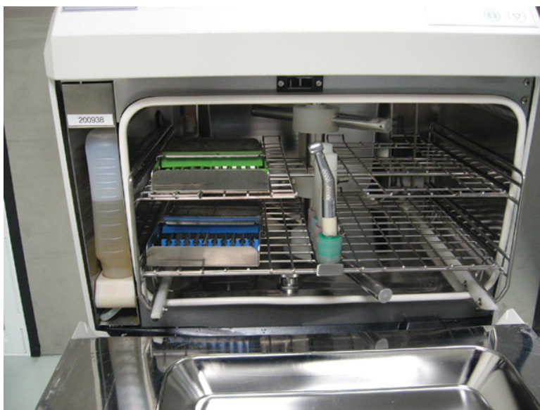
Figure 7.13 Handpiece connectors in a thermal washer disinfector. If the connector is fitted with a filter, these require regular cleaning.
