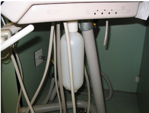
Figure 9.3 Independent bottled water system integrated into a dental chair.
