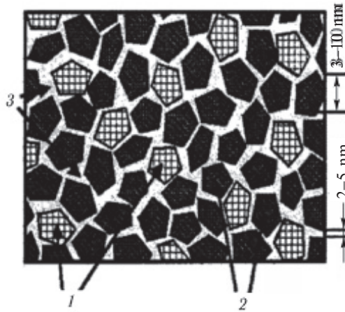
Fig. 3.112. Schematic representation of the nanostructure of the tribological coating: 1 – solid nanocrystals of oxides (nitrides, carbides); 2 – amorphous or nanocrystalline inclusions of Mo or W sulphides; 3 – amorphous matrix (oxides, gold or carbon) [3.244].
