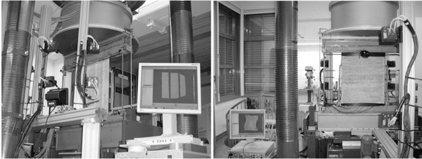
Fig. 11.5 Stationary ultrasonic equipment ( left ) and ultrasonic test setup for cylinders ( right )
