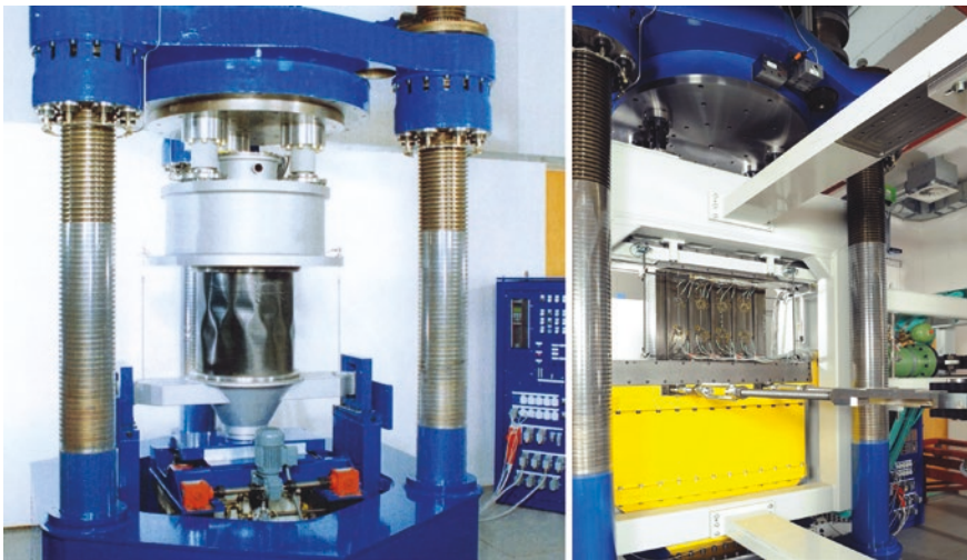
Fig. 11.2 DLR's buckling test facility, axial compression configuration ( left ), compression-shear-configuration ( right )
