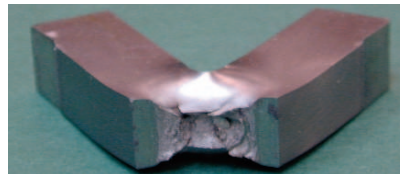
Fig. 2. Incomplete fracture of Charpy sample of high-strength steel
