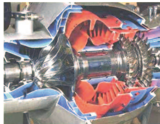
Fig. 1. Sectional view of a typical plane engine illustrating external envelope, compressor, combustion chambers and propulsion turbine [9]
