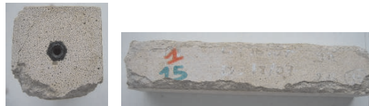
Fig. 8. Photographs of a mortar sample subjected to cycles of immersion-drying at 105°C at the end of test
