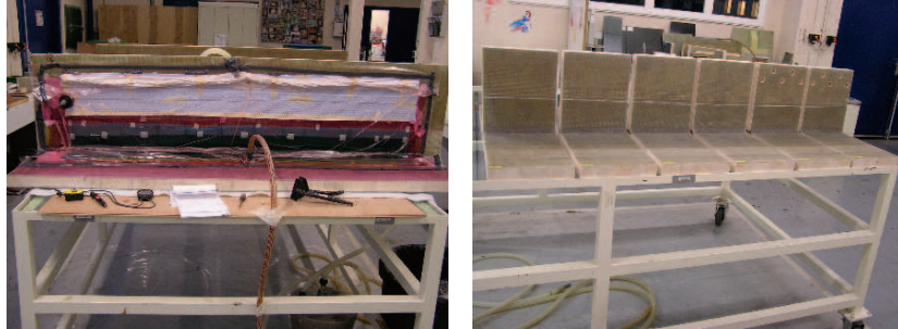
Fig. 2. Manufacturing of T-joint
