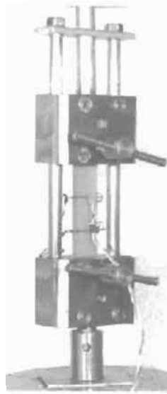
Fig. 3.52. Test fixture for transverse tension and compression of unidirectional strips.
