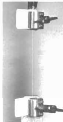
Fig. 3.33. Testing of a microcomposite specimen gripped at the ends.
