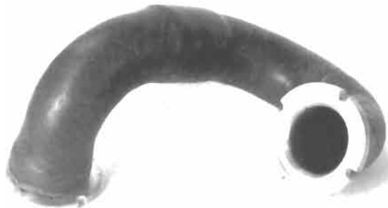
Fig. 4.64. A curved angle-ply pipe made by deformation of a filament wound cylinder.
