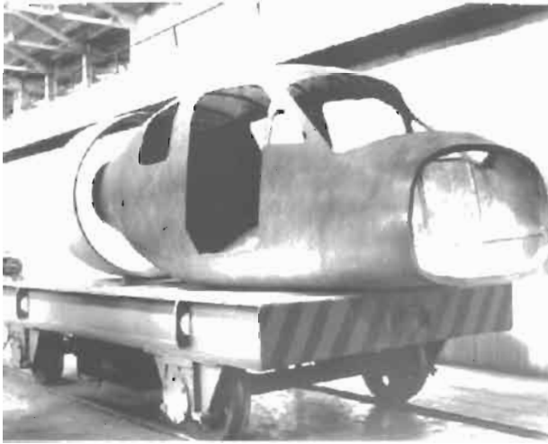
Fig. 1.21. A body of a small plane made by filament winding. Courtesy of CRISM.
