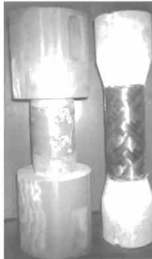
Fig. 6.20. Segments of composite drive shafts with test fixtures. Courtesy of CRISM.
