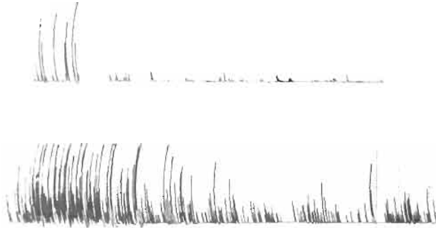
Fig. 4.54. Intensity of acoustic emission for a cross-ply two-matrix composite (above) and a traditional fiber-glass composite (below).
