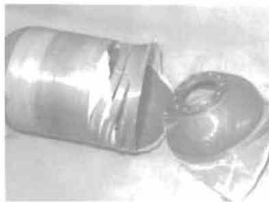
Fig. 6.23. The failure mode of a composite pressure vessel.
