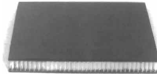
Fig. 5.15. Composite sandwich panel with honeycomb core.
