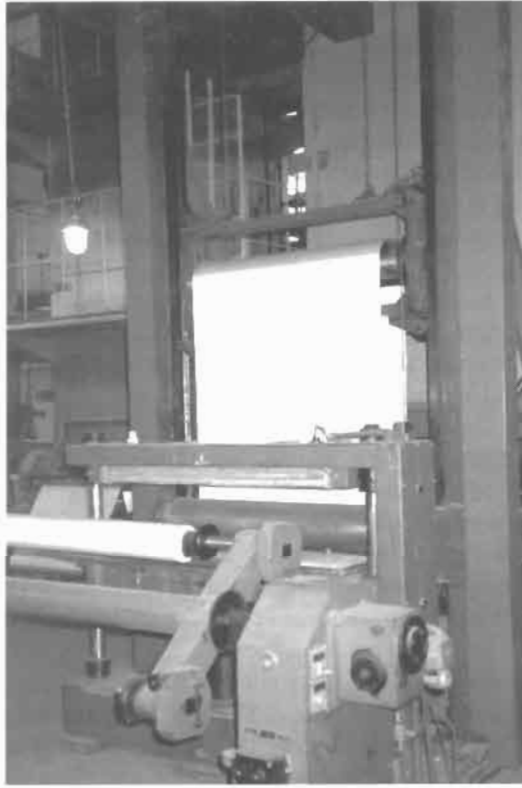
Fig. 1.16. Machine making a prepreg from fiberglass fabric and epoxy resin. Courtesy of CRISM.
