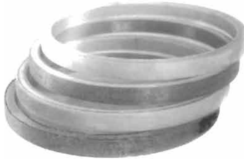
Fig. 5.16. Composite sandwich rings with foam core.
