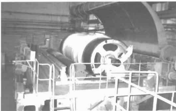
Fig. 1.19. Manufacturing of a pipe by circumferential winding of preimpregnated fiberglass fabric. Courtesy of CRISM.
