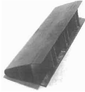
Fig. 4.79. A composite leading edge of an aeroplane wing made of carbon fabric by lay-up method. Courtesy of CRISM.
