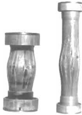
Fig. 6.12. Failure modes of a unidirectional glass epoxy composite under longitudinal compression.
