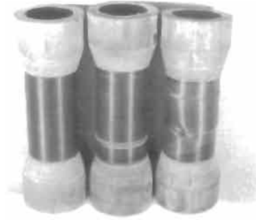
Fig. 6.4. Carbon epoxy test tubular specimens made by circumferential winding (the central cylinder failed under axial compression and the right one – under torsion).
