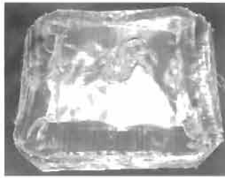
Fig. 7.40. Back view of plate No. 3 (see Table 7.2) after the impact test
