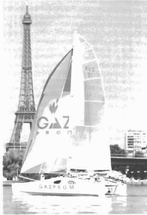
Fig. 1.18. Catamaran yacht Ivan-30 made from carbon epoxy composite by hand lay-up. Courtesy of CRISM.
