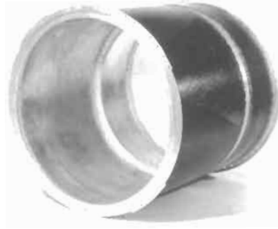
Fig. 7.3. A composite section of a space telescope. Courtesy of CRISM.
