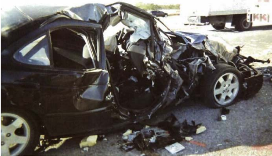
FIGURE 11.7 Right side view of sedan after it was towed away from the trailer, showing extensive damage to the front passenger compartment.
