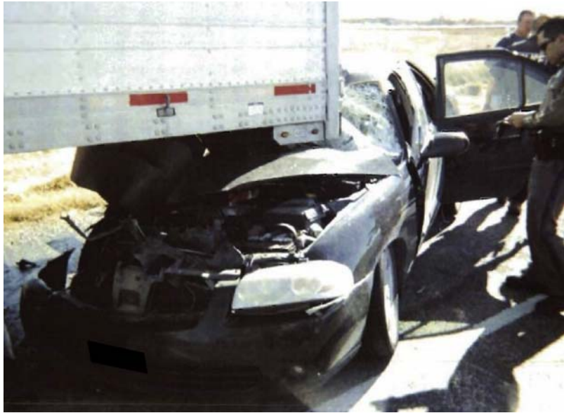
FIGURE 11.5 Left front view of the sedan in full engagement with the trailer.
