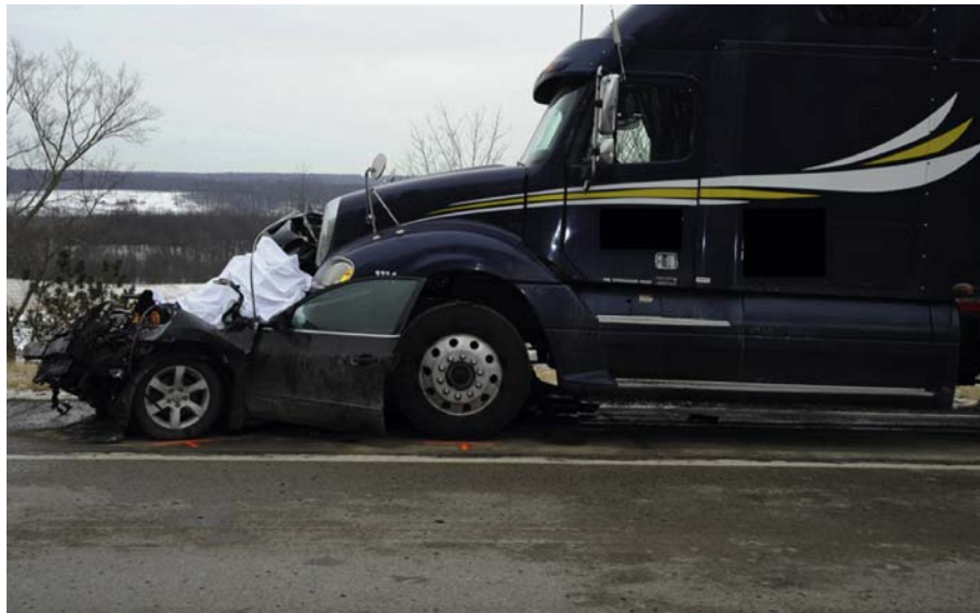
FIGURE 11.1 The semi-tractor/trailer and sedan at final rest. The rear tires of the sedan are obscured by the front tires of the semi, which have ridden up over the rear of the car.
