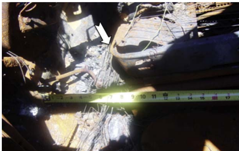
FIGURE 15.2 Photograph of the driver's side foot well with a measurement depicting the distance from the front of the seat frame ( white arrow ) to the end of the foot well. There are approximately 7 inches (0.2 m) of space for the legs of the occupant.
