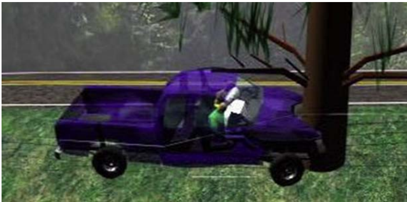
FIGURE 15.6 The point of maximum engagement with the tree and maximum crush to the front of the pickup. Both airbags have deployed. It is at this point that the foot well of the driver is crushed toward the driver (see Fig. 15.2), presenting increased risk of lower extremity fracture. The foot well on the passenger side is preserved (see Fig. 15.3).
