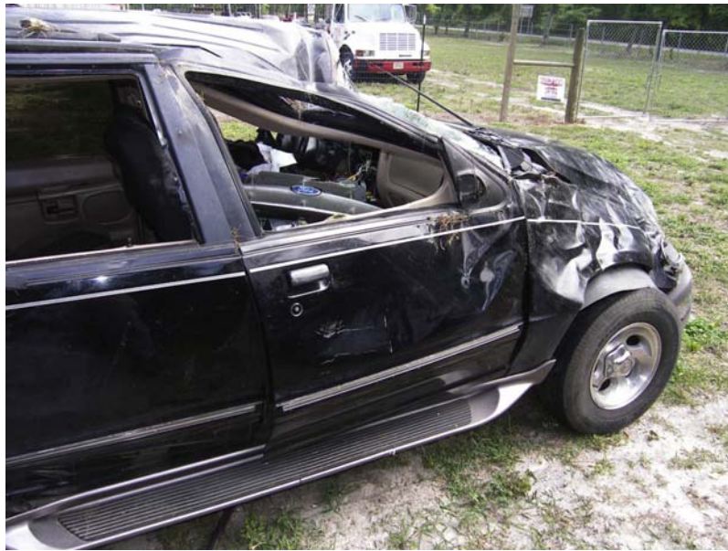
FIGURE 12.4 Passenger side view of Ford Explorer in rollover case study, showing moderate level of vertical intrusion from the roof crush into the passenger compartment.
