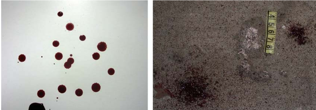
FIGURE 8.21 Drip stains caused by: (left) individual drops from bloodied fingers falling 10 cm onto paper and (right) a series of drops of human blood falling 2.5 m onto concrete, splashing in the pools left by previous drops to create many satellite stains. Courtesy Matt Noedel, Noedel Scientific.
