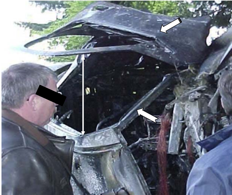
FIGURE 15.4 The induced crush resulting in outward bowing of the driver's side door ( upper arrow ) and driver's side windshield pillar ( lower arrow ) formed a large opening and potential ejection route for the driver between the windshield and the door. The space indicated by the double arrow is ~2 feet (0.7 m).
