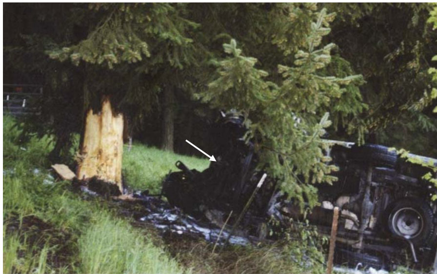
FIGURE 15.1 The vehicle at final rest on its passenger side. The arrow indicates the extensive crush to the left front of the vehicle.
