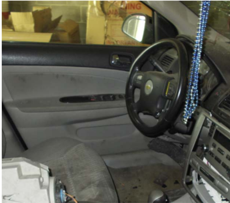
FIGURE 12.2 Interior view of the vehicle, showing the forward deformation of the steering wheel both above and below the air bag cover.
