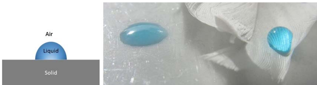
FIGURE 8.15 Surfaces exist between air and water, and between water and solid: at each of these surfaces, there is tension (left). Drops of colored water on a porcelain surface (hydrophilic) and on a feather (hydrophobic) (right).
