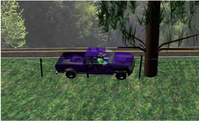
FIGURE 15.5 Right side view of the pickup and tree just prior to impact. Preimpact speed was reconstructed to 55 mph (88 km/h).
