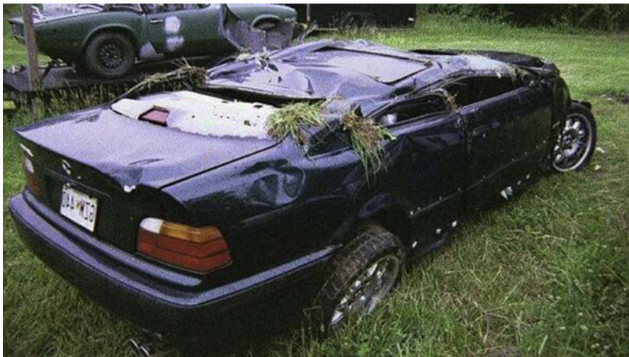
FIGURE 12.3 Example of vehicle with extensive roof crush following a rollover crash.
