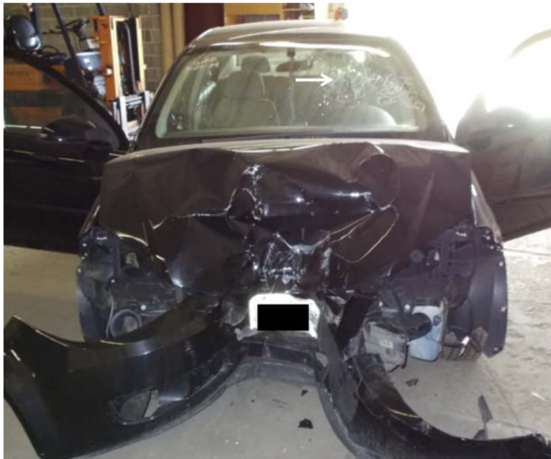
FIGURE 12.1 The front view of the Chevrolet, demonstrating the midline frontal configuration of the impact, as well as windshield damage consistent with a head or face impact ( white arrow ).
