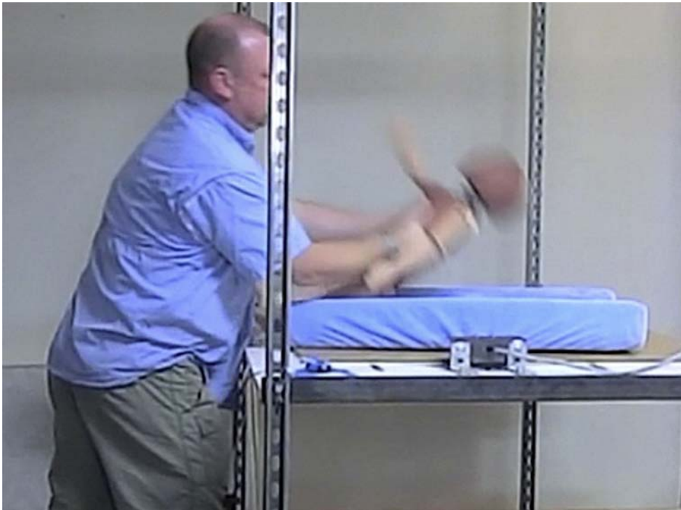
FIGURE 9.11 CRABI-12 mannequin impacted onto changing table pad.
