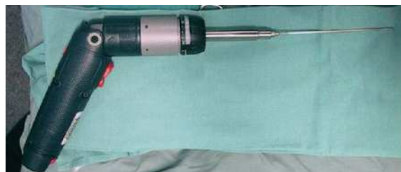
Fig. 8.12. An air-powered drill that can be attached to a biopsy needle
