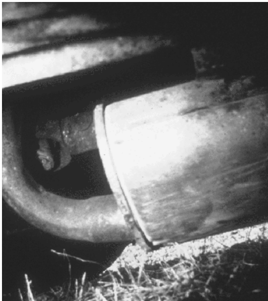
Figure 127 The tailpipe was bent up to fit into the hole.
