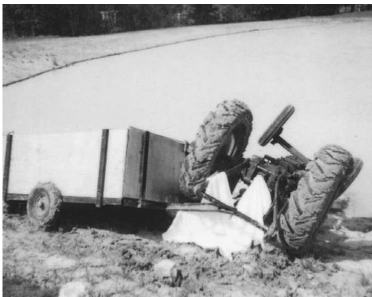
Figure 94 This tractor overturned as it was pulling the trailer full of rocks up the embankment. See next photo.
