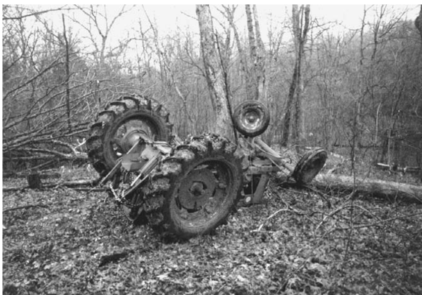
Figure 90 A man was attempting to pull a log out of the woods when the log became caught and the tractor was pulled over backwards. See next photo.
