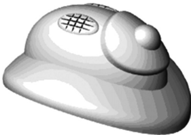
Fig. 13.14 Refillable episcleral explant design forms a seal on the tissue without tight suturing. Bottom surface has opening to allow injected fluid reservoir to maintain direct contact with the sclera. Reprinted from de Carvalho et al. (2006). Copyright 2006 Association for Research in Vision and Ophthalmology. Reproduced with permission of INVESTIGATIVE OPHTHALMOLOGY & VISUAL SCIENCE in the format Other Book via Copyright Clearance Center
