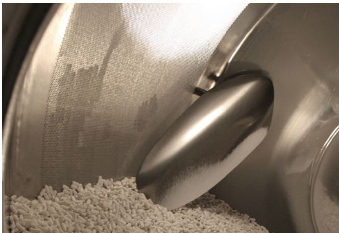
Fig. 3 A film-coating pan containing a bed of tablets (Image courtesy of GlaxoSmithKline)
