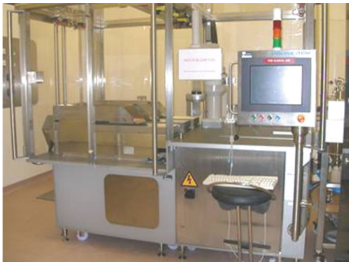
Fig. 5 Pilot-scale production equipment for the GSK polypill technology (Image courtesy of GlaxoSmithKline)
