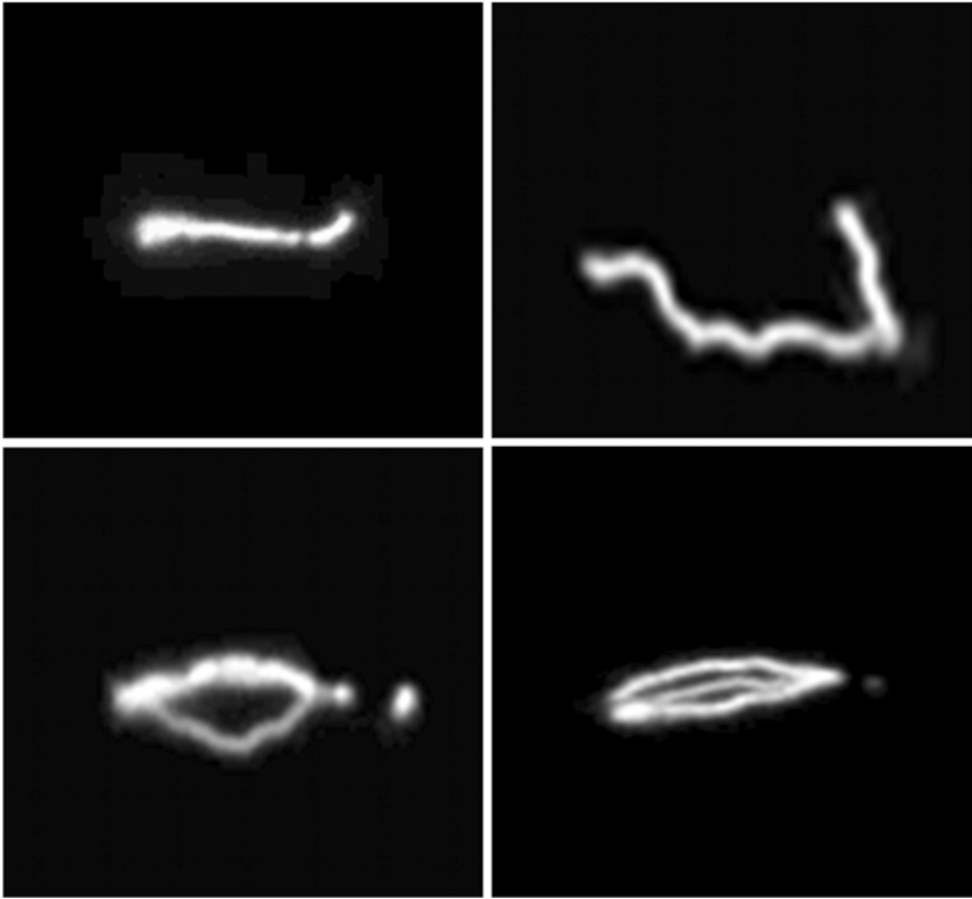
Fig. 4.13 Forms of the discharge channel [39]
