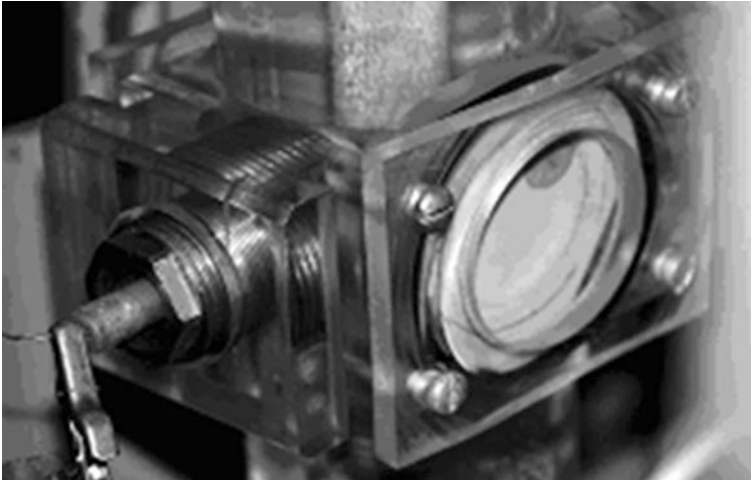
Fig. 3.5 Electrodischarge chamber with quartz windows
