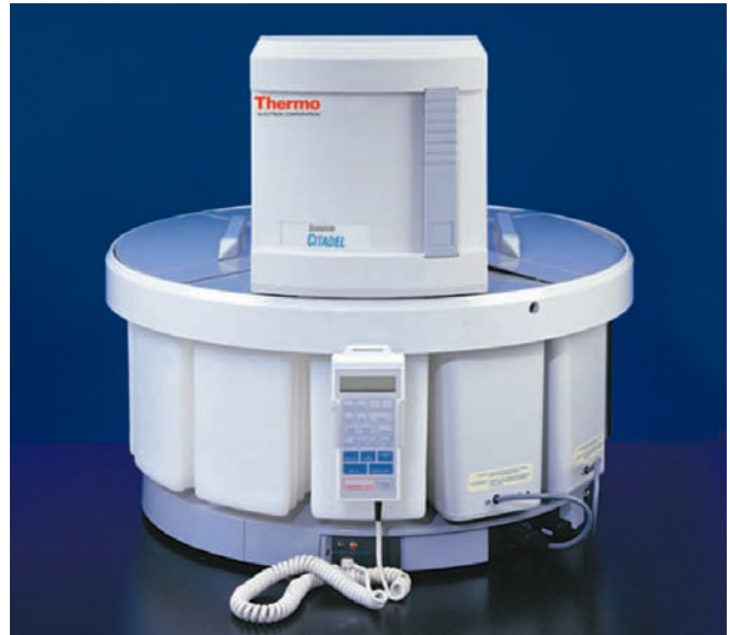
Figure 2.1 ◆ Automatic tissue processor for processing by paraffin-embedding technique. (Thermo Shandon, UK). Courtesy: Towa Optics (India) Pvt. Ltd., New Delhi.
