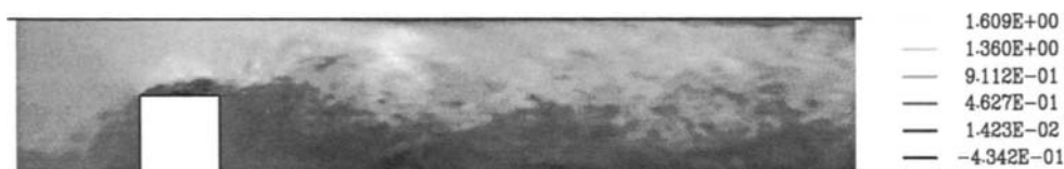
Figure 5. Instantaneous contours of streamwise velocity component u in a vertical cross-section. Velocities have been scaled with U_m .
