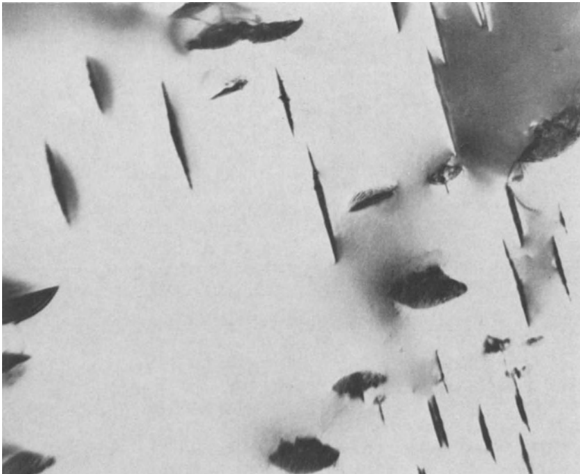
Fig. 5. A transmission electron microscope photograph of coherent precipitation in Pd-Hx at a temperature of approximately 90K. The coherent precipitates (of \alpha -phase in \beta -phase) are the lenticular shapes with almost vertical direction. Some of these, and almost all the thicker precipitates, directed more or less horizontally, have become incoherent, with very high dislocation densities ( \sim 10^{12}/\text{cm}^2 ). The precipitates (average length \sim 1 micron) have their long axes in \langle 100 \rangle directions. For more details, see Ho et al. 21
