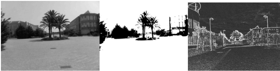
Fig. 4. (a) Grey scale image, (b) Binarization of a scene and (c) Kirsch's filter
