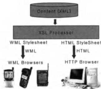
Fig. 3. How XML content is converted to HTML or WML
