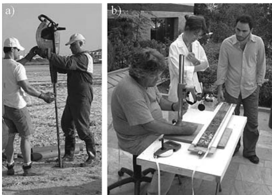
Figure 9. (a) Drillings for the collection of core samples of sediment, (b) Stratigraphic study of the core samples, © Vassilopoulos & Evelpidou 2007.
