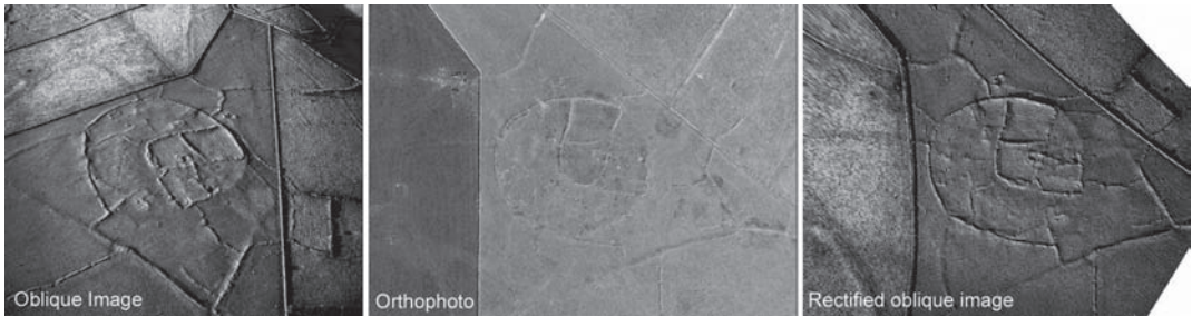
Figure 7. Example of the rectification process of detailed oblique aerial imagery to orthoimagery of the same local.
