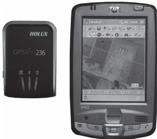
Figure 1. Personal Digital Assistant (PDA) and GPS external device linked via Bluetooth protocol.
