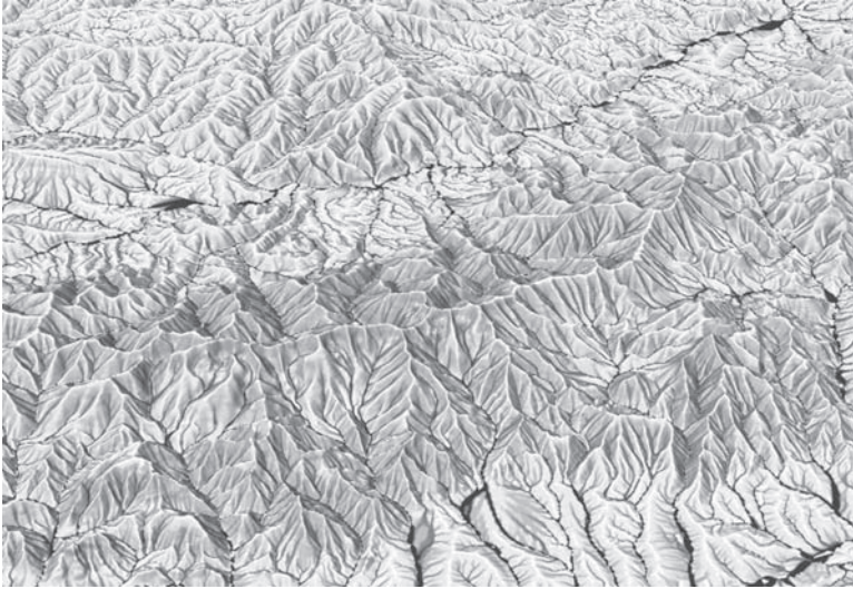
Figure 4. Flow accumulation (in dark grey) draped over the land surface computed using the r.terraflow module in GRASS GIS.
