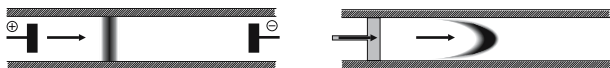
Figure 9.11. Streaming profiles of liquids either pumped mechanically ( right ) or moved by means of electroosmosis ( left ). Parabolic deformation of sample zone is largely avoided with electroosmotic conveyance
