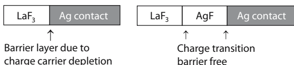
Figure 7.5. Barrier-free direct contact at lanthanum fluoride electrode
