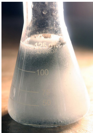
Hydrogen peroxide solution decomposing into bubbles of oxygen in the presence of a black catalyst (manganese dioxide) [Chemistry Land CHM130LL]
