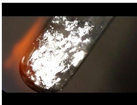
Boiling mercury showing colourless vapour [Taofledermaus, YouTube]
