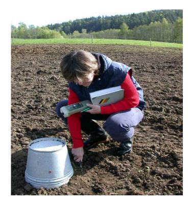
Figure 3. Flux and soil temperature measurements at the cattle overwintering area in 2004. The figure shows the chamber deployed to the severely impacted part of the area. The chamber covers ca  $0.076 \text{ m}^2$  and its volume is ca 15 dm<sup>3</sup>. Notice the soil surface damaged by the animals.
