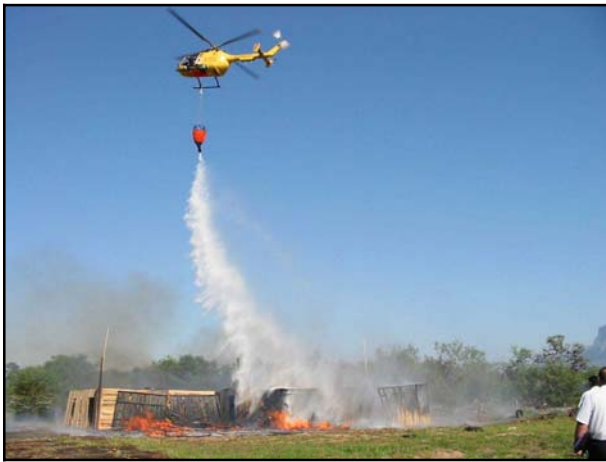
Fig. 11.1. Testing the efficacy of using a helicopter to control fire in a mock informal settlement
